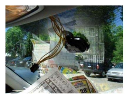
Step 24: Use some silicon spray or other on the track to help the mirror install on. With the wires hanging through the empty space, slowly, SLOWLY, inch the mirror up the mount. ONLY PULL UPWARDS ONTO THE MOUNT. DO NOT PUSH OUT ONTO THE WINDSHIELD.
