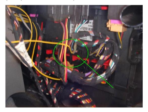
Step 19: Tap Power, mirror is 5A switched, rain sensor 5A unswitched Connect #7 to the Mirror, #17 to the Rainsensor.
