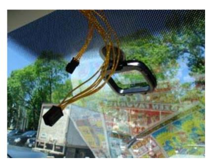
Step 12: If you look at the blue connector, you'll find an open connection! Connect wire 6 from the mirror into here and the mirror will not darken when the interior light is on.
