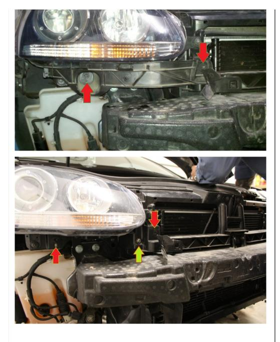
Remove the top outer bolt on each side of the metal bumper (16mm socket). Replace each of these bolts with the M10 x  $1.5 \times 120$  bolts (red arrow). Remove the remaining three (3) bolts on each side (green arrows).
