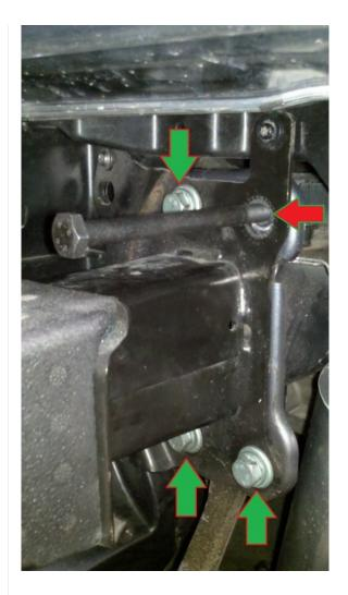
Now slide out the lock carrier and separate the radiator and friends from the lock carrier and place on jack stands. Take out the long M10 bolts and move the lock carrier out of the way. You might find it helpful to disconnect the intercooler hoses. You might even consider removing the intercooler entirely.
