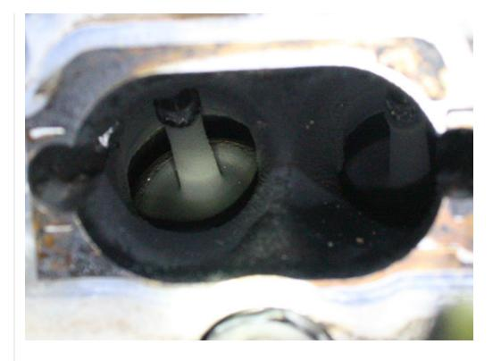
Now take the plastic baggy and cut decent sized pieces out of it. Cover the ends of the injectors and wrap twist-ties around the plastic behind the blue o-rings to keep it on there and kinda seal it off a bit. Now lay some paper towels or shop towels over the injectors. Do your best to keep the towels up against the block when you're cleaning so crap doesn't fall down on the injectors and stuff. \*NOTE: This picture was taken after cleaning, so it WON'T look this clean.\*
