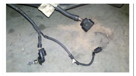
On both sides of the car, unplug the headlights, airbag sensor things, and then the hood latch sensor on the passenger side by the other plugs.
