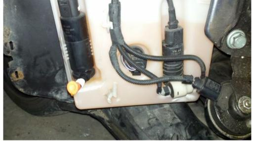
Unplug the fogs and side markers. Also, unplug the fog light wiring harness. It's that plug dangling above the fog and sidemarker wires in the picture. To find it, follow the fog light wires up into the engine compartment on the driver's side.
