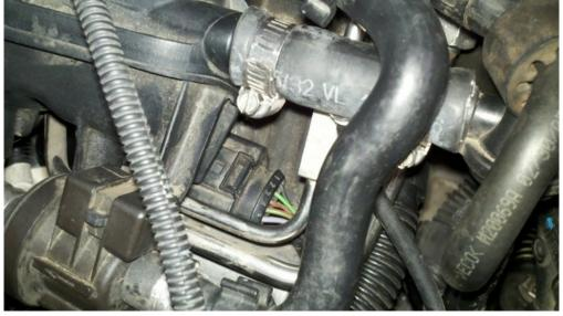
Next, I removed my catch can and plugged the holes with paper towels. If you have the stock PCV setup, I don't know just how in the way it is, but I do know that you'll have to disconnect some hoses. Also, unplug the breather hose to the left of the PCV/catch can area. Also also, remove the nut holding the coolant line to the left of the intake manifold. Now take out the circled T30 bolts.
