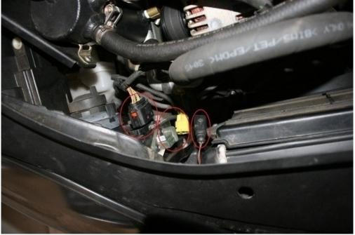
Disconnect the hood latch popping cable right above the driver side headlight. If this is the first time you've done it, it will be pretty hard. Use a screw driver to pry up on the side.
