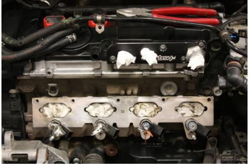
If you have injectors in the intake manifold, pull them out, reseal them (if you don't have new resealing kits, then you can just carefully put them back in the block and hope for the best), and put them back in the block. You might consider vacuuming out the hole the injector(s) go into. Mine had some dirt or something in there. Below is a picture of a properly resealed and ready-to-be-reseated injector.
