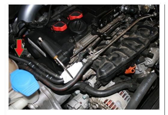
You're going to need to remove the throttle pipe. To do so, loosen the hose clamp connecting the throttle body hose to the throttle body. Undo the bolt securing the throttle pipe. Unplug the sensor in the pipe. Disconnect the intercooler hose, if you haven't done so already. Now yank it out! Also, unplug the circled sensors.
