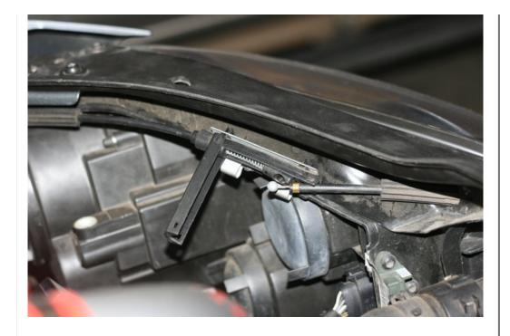
Remove the 2 torx bolts on the top of the lock carrier on both sides (above the headlights). They're T30 bolts. Don't remove the screws for the headlights.
