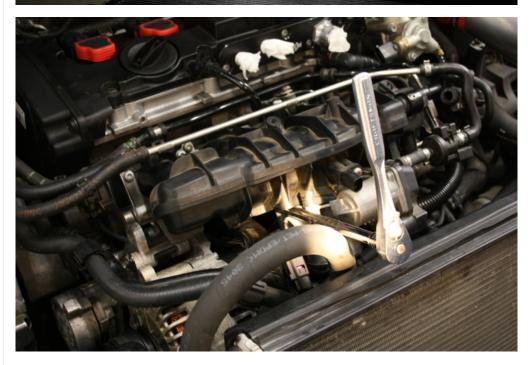
Now there are some wires you need to unplug under the intake manifold. Below is a picture of the wiring harness. Before you read this section and get all antsy in your pantsy, go ahead and put some rags or paper towels under the fuel rail, which is directly below the intake manifold itself. Basically, just put some rags under the manifold. When you start pulling out the manifold, if injectors stay in the block, some fuel will pour out of the rail.
