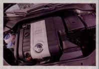
>> A competent handler at the track, the GTI is really in its element on winding back roads, where its chassis delivers comfort, compliance and composure. Much credit for its strong performance numbers goes to the 200-bhp 2.0-liter turbocharged four, above, which enjoys the broadest powerband of our trio, plus the advantage of quick and seamless shifts from the optional 6-speed DSG transmission. The hatchback styling, left, may not be especially inspiring, but its functionality is tough to beat.
