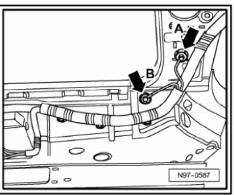
45 - Ground Connection (behind instrument panel, center)  $\Rightarrow$  - Arrow-
