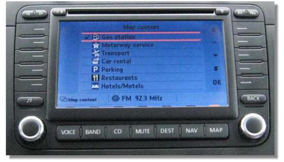
From the "Map" screen you can also select the compass which tells you lat/long, elevation, current heading, and straight line bearing/distance to destination.
