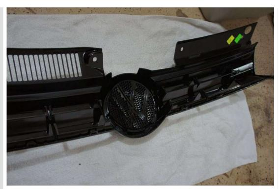
**Step 5.** These are the two fused tabs. They need freedom. The top tab is normal and secured with just the working tab.
