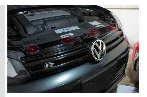
Step 3. Pull the grill up and out. Each side needs special attention. Grasp the lower bar and pull out next to the headlight. It seems as if it will break but it just pops out. Pushing down on the bumper seems to help.
