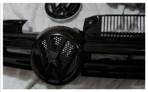
Step 9. Reinstall the grille. Just put the lower end in first and pull the top forward. A little snap can be heard. Replace the screws. You are done.
