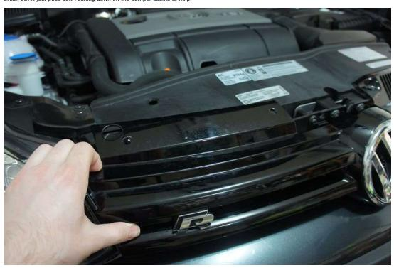
$\textbf{Step 4.} \ \text{Rest the grill down on a non abrasive surface. Three tabs hold the emblem onto the grille.}$
