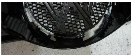
**Step 8.** Pop the new emblem on slightly counterclockwise to line up the top tab and then rotate it clockwise. The bottom two tabs actually latched for me. They did not follow the traditional lip but secured nonetheless. Minor repositioning got it perfectly center. It was secure enough that no adhesive was required.
