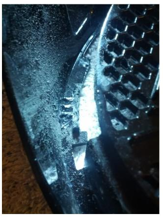
Once the bottom two clips are loose, the top clip can be undone by swinging the bottom edge of the emblem out and up:
