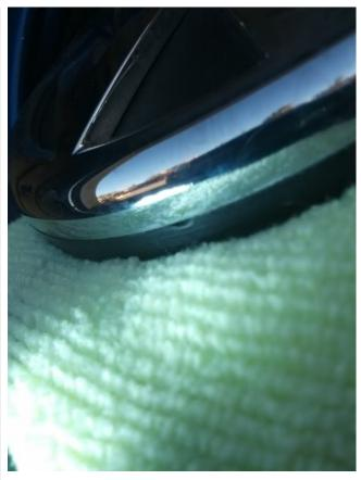
Carefully pry outward with a small screwdriver and/or razor blade. Do NOT twist the screwdriver or you will put dents in both the emblem and the handle. Do not sink the razor blade too deep into the handle -- only use the thickness of the blade to push the emblem off the handle. Start at the bottom and work your way up both sides. When you get to about half way up, work on the V and W. It should pop off then.
