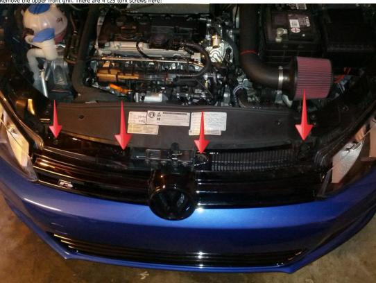
Then pull BOTH lower corners straight out **at the same time**. There are several clips holding the bottom edge of the upper grill to the bumper cover, but the majority of the 'grip' is in the lower corners:
