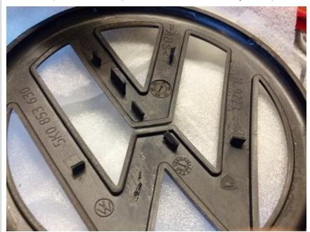
I added a dab of RTV to the clips to prevent vibration from knocking it loose.
