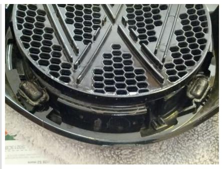
Grind away at the plastic with a dremel tool or file until the emblem can come loose from the grill. Be careful not to go too deep or you could come through the visual portions of the grill on the front side.
