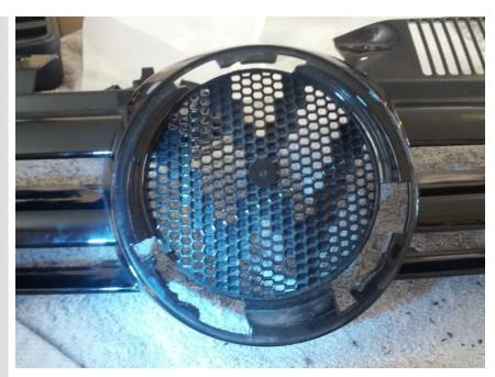
Place the new emblem into the grill. It will have to be at a slight angle, tilted to the left from looking at the front.
