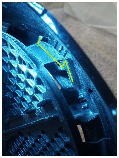
However, the bottom two clips have been melted. You can see where the ramps and cups should have been underneath the melted areas:
