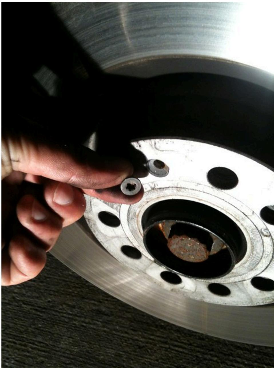
Benz rotor "set screw" hole, see the difference? There isn't a tapered hole that's anywhere close in size to stock.
