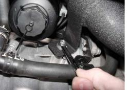
Use WD-40 or equivalent to lubricate inside of upper rubber hose to ease pipe installation. Install NEUSPEED pipe from underneath and insert into upper rubber hose. Attach mount with supplied M6 x 20mm flange hex bolt. Do not tighten clamp at this time.
