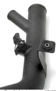
Transfer boost sensor to NEUSPEED pipe using supplied M6 x 16mm hex key bolts (electrical connector faces upward) and install the original rubber grommet and steel sleeve to bracket.
