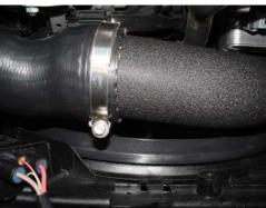
7. Again, use WD-40 or equivalent to lubricate inside of lower rubber hose to ease pipe installation. Attach lower rubber hose to NEUSPEED pipe. Check alignment of NEUSPEED pipe and tighten both upper and lower hose clamps.
