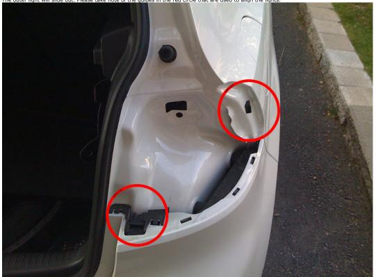
Once the new LED light is installed, hand tighten the white screw. Then plug the connector that was plugged into light where the green box was and plug it into one end of the LED Adapter. Then plug the other end of the LED Adapter to the LED light. It should look like this once completed.
