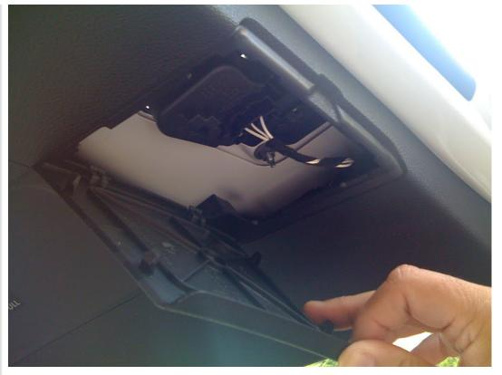
Once opened, you will need disconnect the plug in the green box and then use the 8mm socket or wrench to remove the nuts in the red circles.
