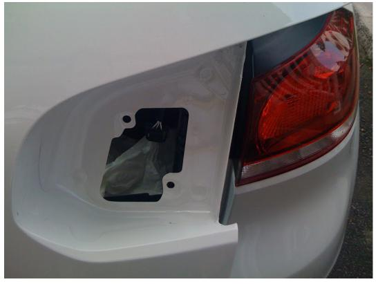
Take the new Inner LED tail light and secure it to the hatch with the same two 8mm nuts.
