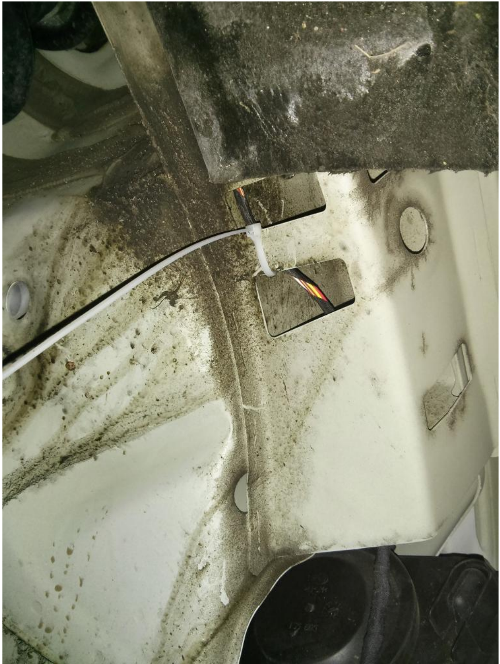
This is the passageway at the top of the wheel arch.
