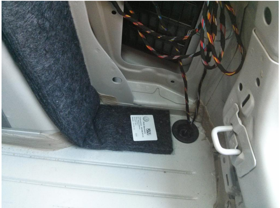
Here is grommet going to the rear bumper.
