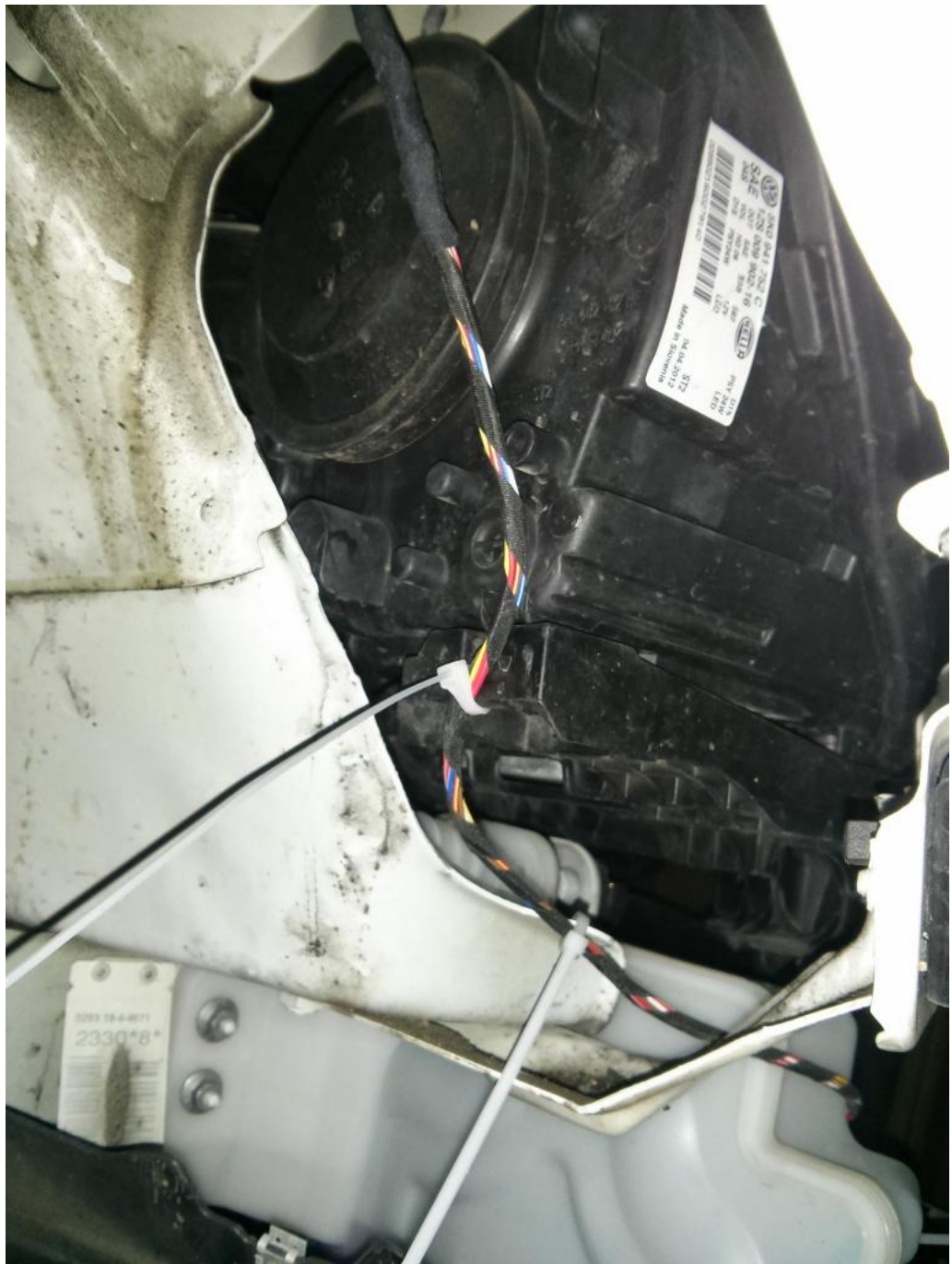
This is the back of the passenger headlight after wheel and all liners were removed.
