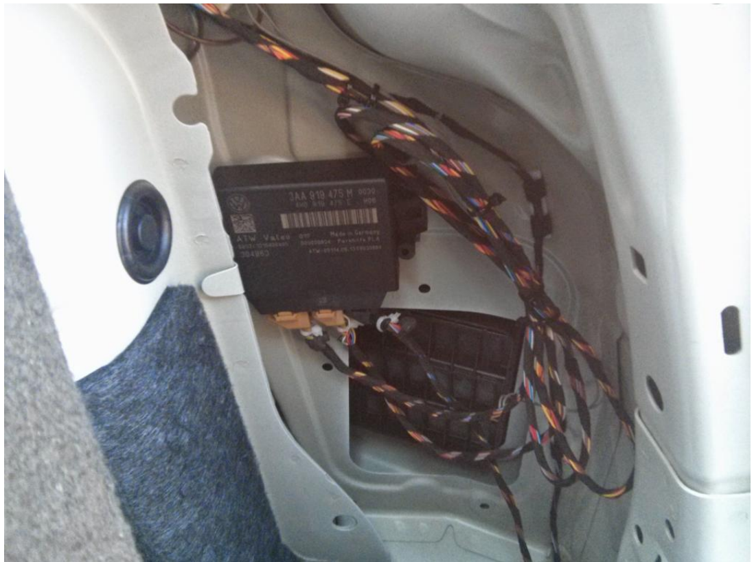
The finished install of the module. (If you have steel fish tape you can fish the wires through the channel above the wheel well.)
