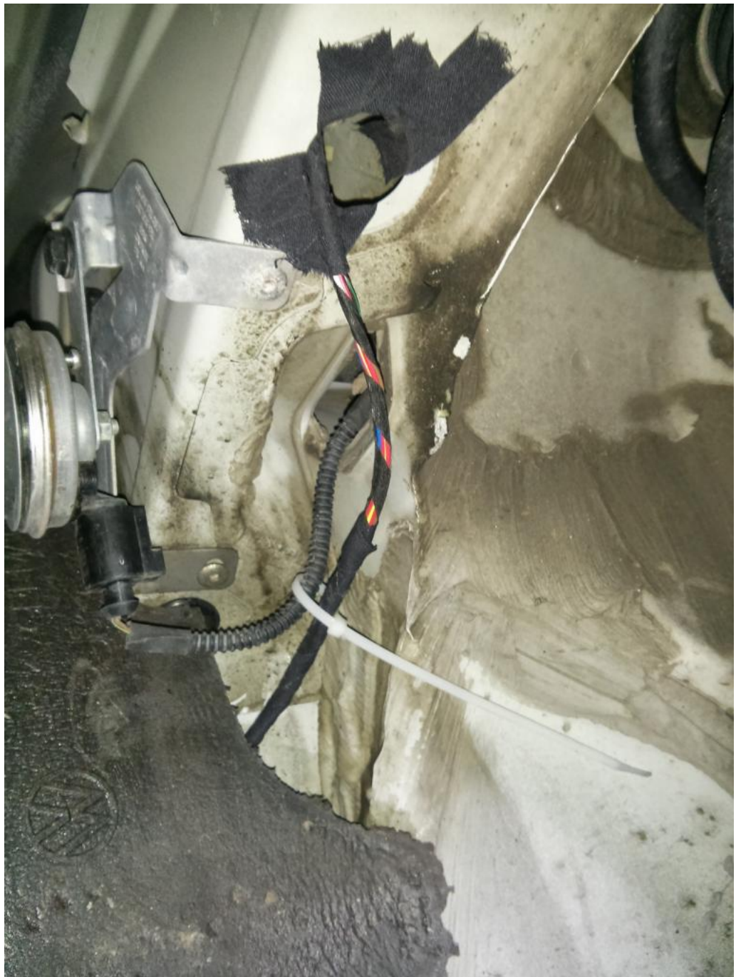
This shows the exit of the passageway and where it goes behind the foam to exit between the fender and body in the door channel.
