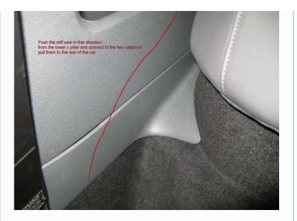
To remove the C pillar covering, remove the air bag tag and remove the torx screw located behind and then remove the trim. I found it wasn't necessary to remove the trim panel as there is enough room to get the cable run up behind if you carefully pull the C pillar trim away from the bodywork by the rear opening
