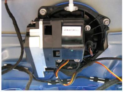
One of the legs of the wiper motor needs to be removed so that it looks like this, the legs are only plastic so it's easy to cut.
