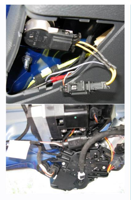
Close the rear door, turn on the RNS510, turn the ignition on and then select reverse gear. You should then see the rear view image on the screen. Selecting forward gear should return the display. If you do not move forward the badge will stay open for several seconds and then close.
