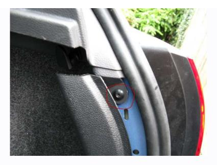
The whole panel can then be pulled out. Take care as the wiring is short. It's held in place by three white studs. Refit the studs back to the panel removed before putting the panel back.
