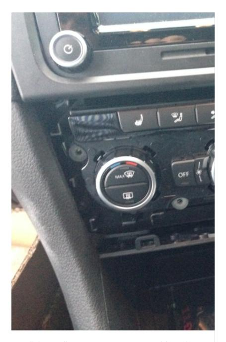
Install the small groove cover you removed from the old fascia into the new fascia. Re-fit the climatronic fascia underneath the RNS/RCD fascia, then re-fit the RNS/RCD fascia above.
