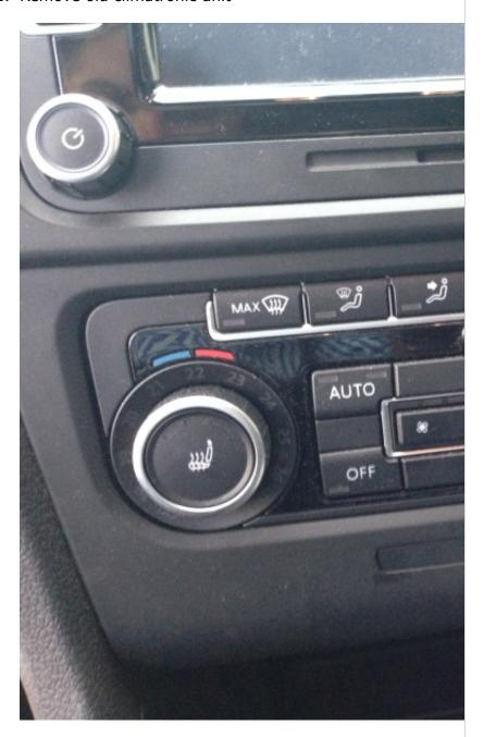
Loosen the fascia at the bottom of your RNS/RCD unit. It doesn't need to come off completely, but loosening it will make re-installing the fascia for the climatronic easier. A small flat screwdriver used from the sides can help get a corner up, but gentle force by hand is the safest way to remove the fascia without scratching it.
