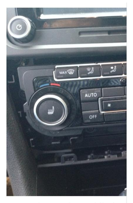
Use a T20 Torx bit to remove the 4 screws holding the climatronic unit in place. Pull it out gently.
