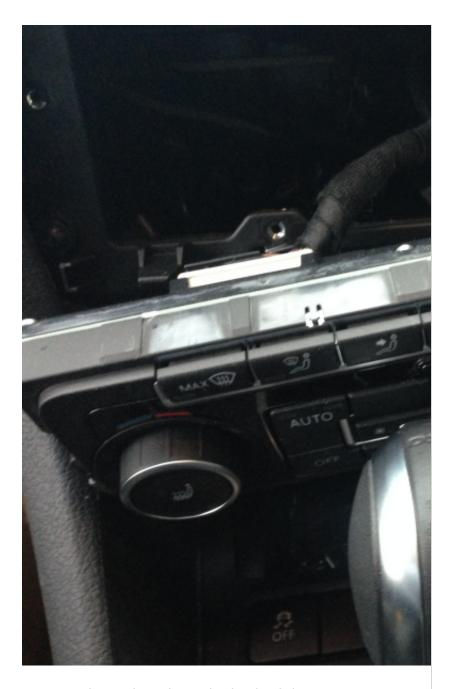
Remove the 3 plugs from the back of the unit. To remove, pull the small red locking pieces upwards (towards the back of the unit), which will allow you to depress the locking tabs on the plugs themselves. Each plug is uniquely shaped so no need to panic if you can't remember which of the small plugs came from which socket.
