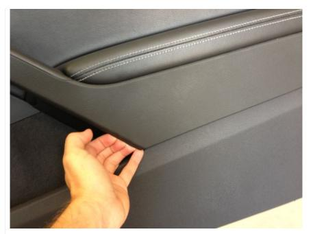
There are about 12 clips that hold this in place. Once the center pops out work your way up the door trim piece and then back down the other side. The part closest to the door latch needs to come out last.
