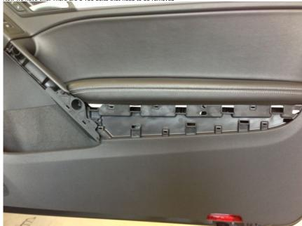
Once you've removed the 3 bolts, you want to pop the door clips off. Be careful to pull straight out quickly and firmly. You can use a trim removal tool here if you feel that is more appropriate. I found it easiest to grab here and pull hard with both hands and that will pops 4 of the clips.
