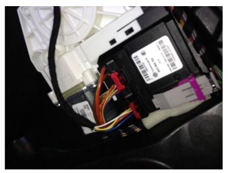
Swap the door controller with the new high line controller and reinstall the door window motor assembly with the 3 T25 screws. Re connect the wire harnesses to the new door controller except the smaller black/red harness. It is the mirror harness.
