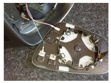
Here are the two clips that hold the black mirror housing trim to the assembly. Release these clips and pull the trim away from the housing.
