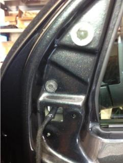
You should now be able to pull the housing away from the car and route the wire harness through the hole in the door frame.
