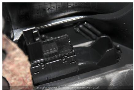
With a small screwdriver, push on the tab that hold the trim in place and pop it off from the top of the door panel:
