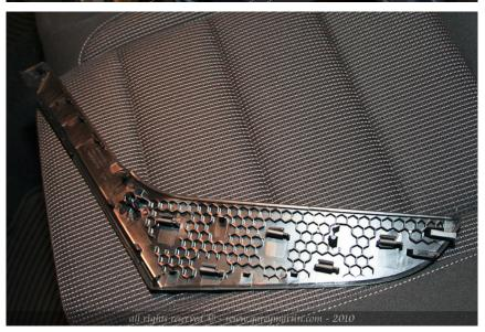
Next, pull the door panel off. It has 6 clips holding it in, 3 on the front part 3 on the rear part, and at the top it slides into the window channel. Once it is loose from the car, unplug 2 harnesses, one from the tweeter in the door and one from the window switch, and remove the cable for the door latch (little tab pulls back and it comes right out) and take the door panel all the way off:
