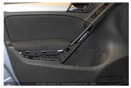
Remove the door panel the same way you removed the rear ones, but remember the driver's door has 4 harnesses instead of 2. Here you can see 3 connectors on the first pic (window switch, door lock switch and mirror switch) and 2 connectors on the second pic (door LED and the mirror switch from the first pic again):
