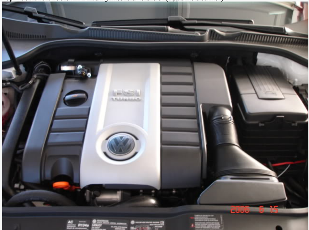
Pop-Hood and unscrew MAF using metric size 3 bit: (upper left corner)
