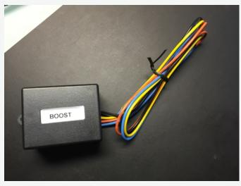
BLACK - connect to a solid chassis ground under the dashboard or directly to the negative terminal of the battery. You
