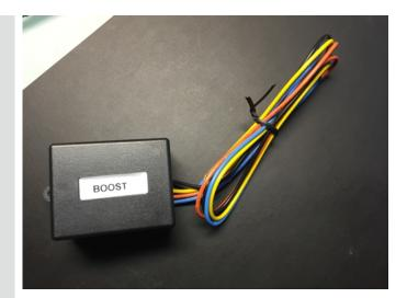
BLACK - connect to a solid chassis ground under the dashboard or directly to the negative terminal of the battery. You may need to expose the metal connection point under the dash by scraping or lightly sanding it.
