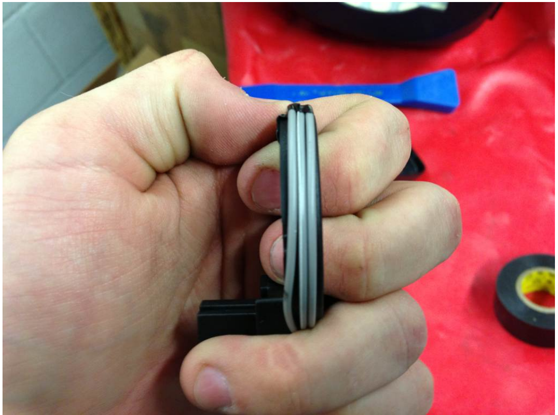
Wrap 3 loops from the other side of the cut valet switch wire. Tape it up.
