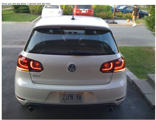
If you have a newer Cent. Elect. Module and using a kit without a reverse lights, you are done. If you have an older module, then you will need the coding box from TMT or use VCDS to change Byte 18.
