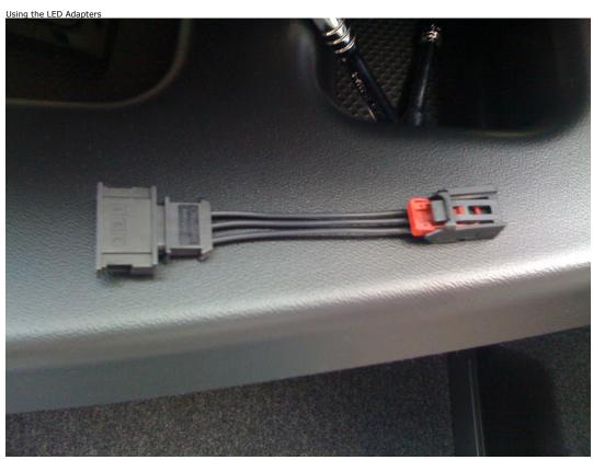
Plug the connector that was plugged into light where the green box was and plug it into one end of the LED Adapter. Then plug the other end of the LED Adapter to the LED light. It should look like this once completed.
