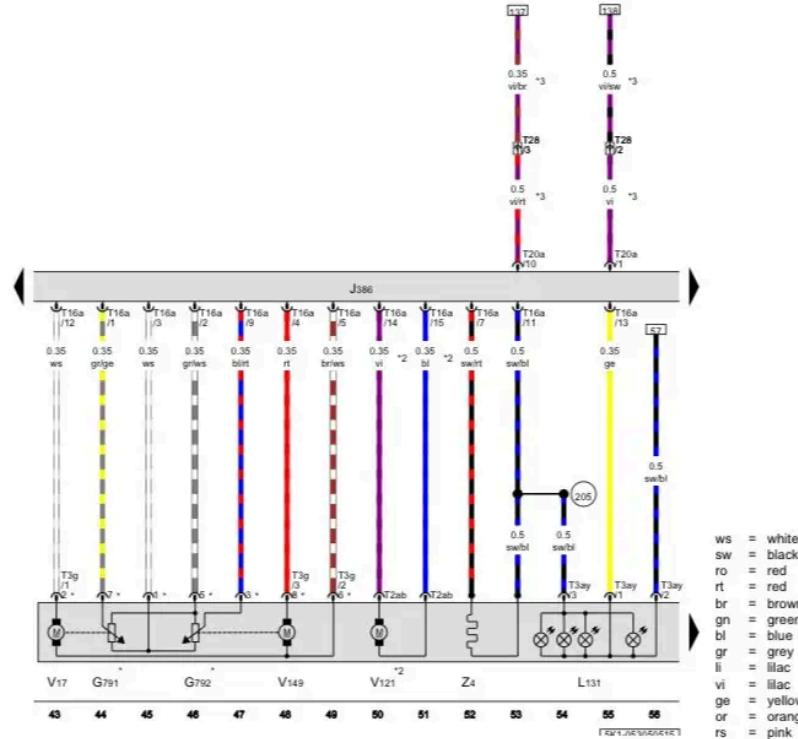
The right side text explains what the call out connection colored wires it says t16a that refers to the 16pin connector
