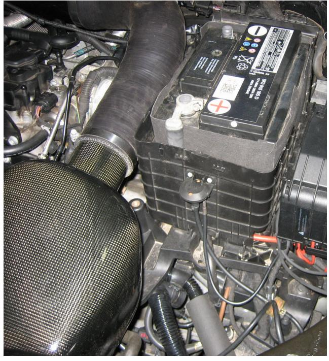
Determine where you're installing your gauge. I opted for Osir's dual pod setup to run oil pressure and oil temperature. Therefore I removed the sthrough. Feed the sender wiring as well as your power/ground wiring through.
