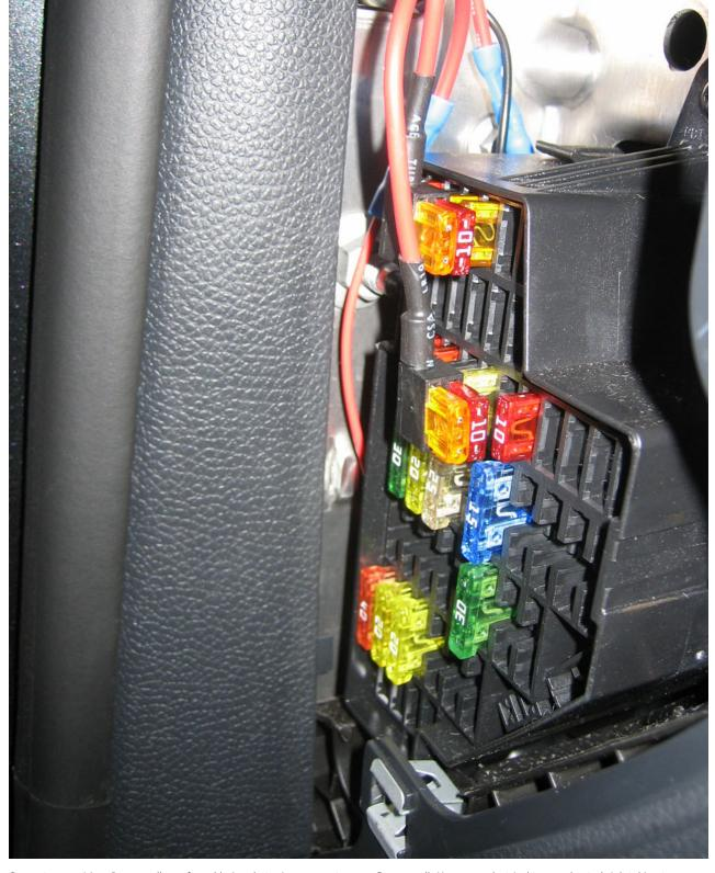
Connect your wiring. I personally prefer soldering, but crimp connectors are fine as well. Use some electrical tape or heat-shrink tubing to cover u layout, for mine:
