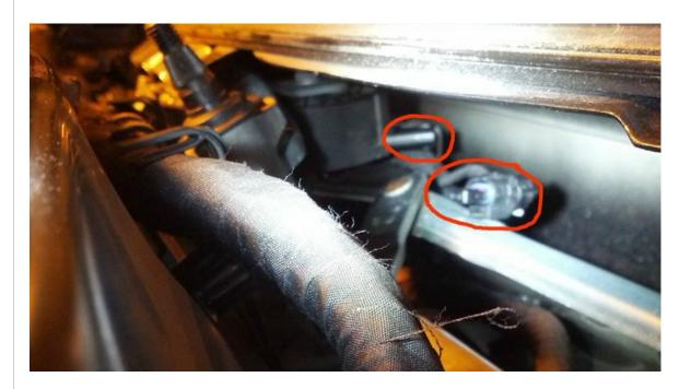
9. This part is up to you. You need to secure the wire and connector so they don't rattle around and get dirty. Since I could barely get my hand in there so securing the connector with a tie or tape seemed like more trouble than it was worth. Instead, I wrapped the connector in plastic and stuffed it under the cable under the soundaktor. Just make sure it won't get wet and dirty and can't get in the way of the wiper assembly when it moves.
