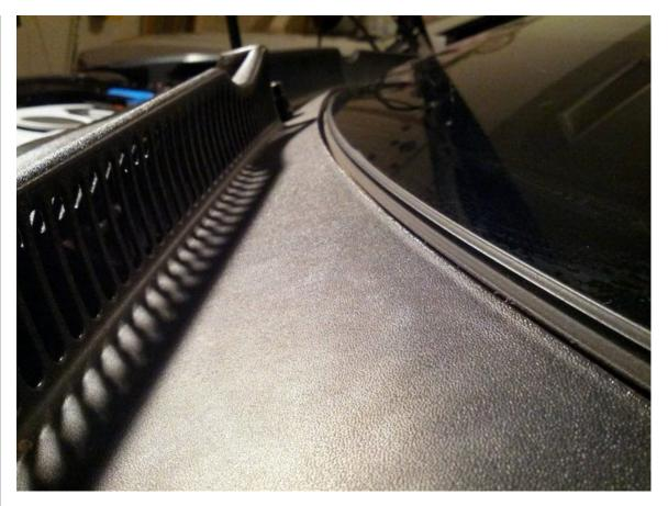
6. Unless you have very small hands, remove two nuts holding the windshield wiper bracket. The Soundaktor is connected to it. This will let you push it down and back so you get your arm in to pull out the connector.
