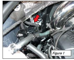
Disconnect the wire harness from the controller by pulling up on the rectangular tab at the top of the connector, at arrow in **Figure 2**.
