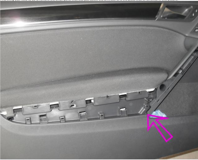
The red arrow indicates where you should start to pry the piece upwards, it starts to pop up pretty easily and you shouldn't have to use much pre Work your way around the piece carefully pulling towards you and slightly upward. Once you reach the rear you should be able to slide it forward. careful not to pull the rear section straight out, as it is looped in behind the main panel and you might break something. Once you have it remove aside.
