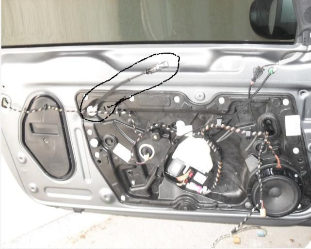
the latch mechanism simply unclip from the panel by pulling on it, and all the wires unclip in a fairly straight forward manner. make sure not to fo about the little blinking red light thingy on the top of the drivers side panel.
