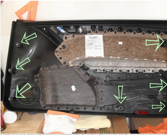
I had the most luck by starting with lower rear corner (bottom right in this pic) then sliding my hands under the panel and slowly moving towards of the car while slightly pulling towards my body. Try not to lift or pull down on the panel, but pull as straight outward as possible. Once you have to the three along the bottom move up along sides remembering to pull straight out.
