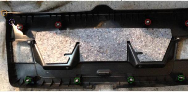
I had some left over lightweight uber-expensive damping from an aircraft that I thought I'd put on there. While I was at it, I buttered up all with white lithium grease:
