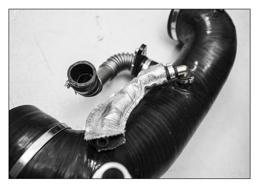
Install vacuum line from boost control solenoid to turbo inlet hose barb, trimming if necessary. Secure with cable tie. Now is a good time to secure all vacuum lines from boost control solenoid together with included cable ties.
