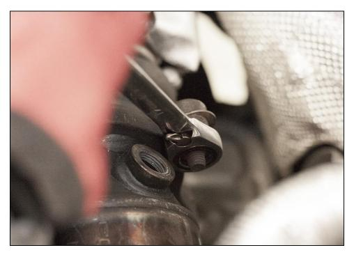
Remove the two bolts holding the exhaust hanger to the subframe using a 13mm socket.
