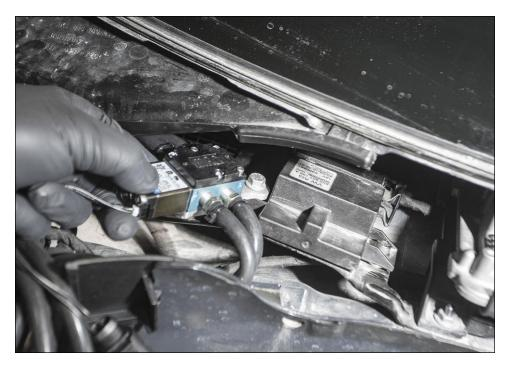
Carefully run all four vacuum lines through plastic grommet. Connect the solenoid harness to the OEM N75 plug. Place harness in grommet with plugs in the rain tray. Slide upper portion of grommet back in to secure all hoses.
