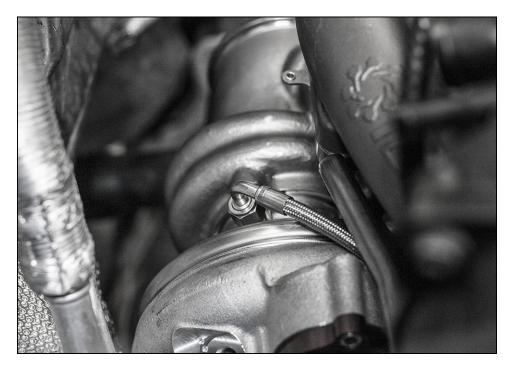
It is necessary to prime the turbo with oil before the first start. This is a good time to do so, using a clean funnel in the feed line. Pour enough fresh engine oil into the line to reach the turbocharger and lubricate internal ball bearings.
