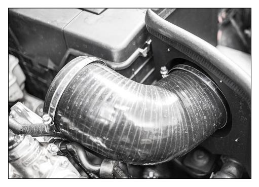
Install straight reducing coupler onto MAF housing. Secure with 90-110mm clamp. Slide 80-100mm clamp onto coupler.
