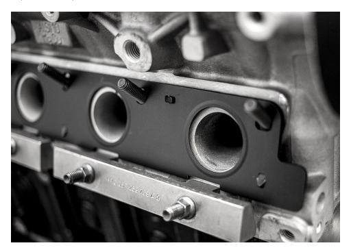
Lift turbo/manifold assembly up and slide into wedge blocks on the bottom side of the head flange. Then, tilt manifold forward with slots over studs. Thread on new lock nuts by hand, five in total. Torque the five nuts on the top side of the manifold to 20 ft/lbs, working from the center out.
