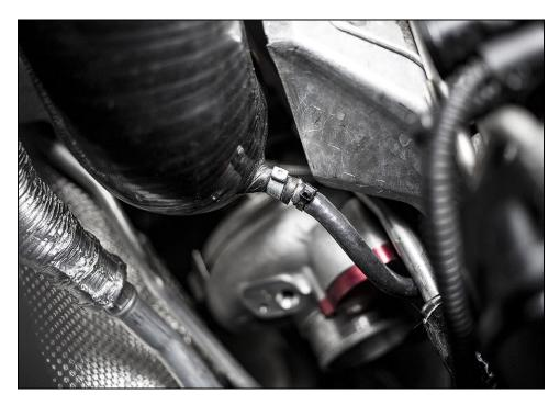
Slide lower clamp onto inlet hose, install pipe onto turbo inlet. Do not tighten clamp yet. Hold MAF housing up to inlet hose and locate mount holes. This is done to orient the inlet hose correctly. Set MAF housing aside and tighten lower clamp.
