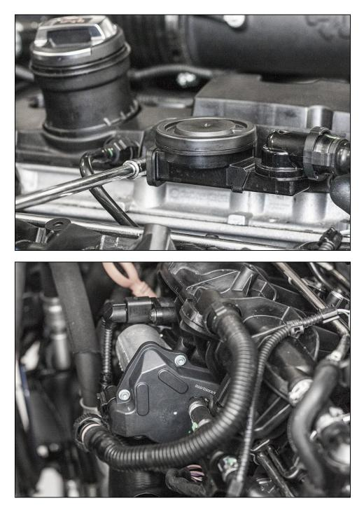
Remove the four screws holding the hard lines to the top of the intake manifold using a T30 Torx socket. This will allow the lines to be moved out of the way to access the rail valve from above.
