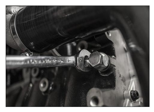
Loosely install coolant feed banjo onto rear port of the turbo with OEM banjo bolt and new crush washers. Slide blue silicone hose onto banjo with clamp on it, then clock line as needed. It should go straight down and run parallel with the oil drain line, then back up to the block. Once clocked properly, you can pinch the clamp, then slide heat jacket over clamp. Install new crush washers and tighten banjo bolt.
