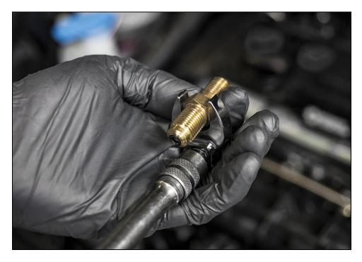
Install new rail valve. It is often difficult to get it started in the fuel rail, but a piece of rubber hose can be slid over the valve to guide it into the fuel rail and get threads started. If using a piece of hose to start the threads, ensure that it is very clean before sliding over valve. Remove hose and tighten rail valve.
