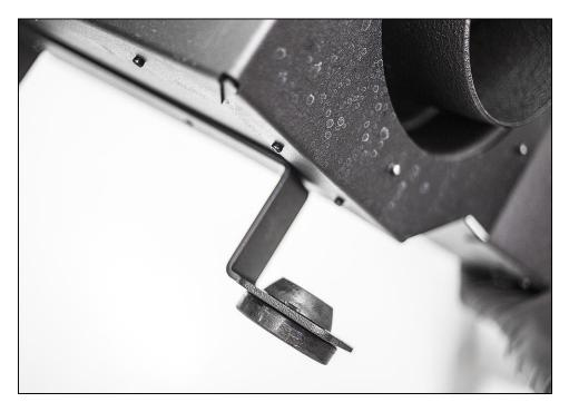
Install heat shield onto plastic pins in front of battery. It may be necessary to use silicone spray to lubricate grommets before installing. Secure mount tab on heat shield to radiator support using factory screw.
