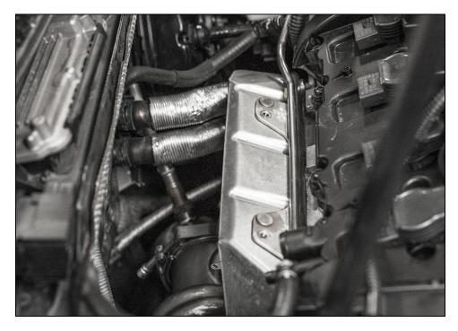
Reinstall 5mm triple square bolt to secure hard line bracket.
