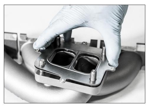
Slide manifold into the turbocharger.
