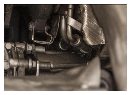
Slide smaller turbo outlet clamp onto coupler with screw facing the rear of the car, on the top side of the coupler. Slide coupler onto turbo outlet. Slide larger clamp onto opposite end of coupler and slide in turbo outlet pipe.
