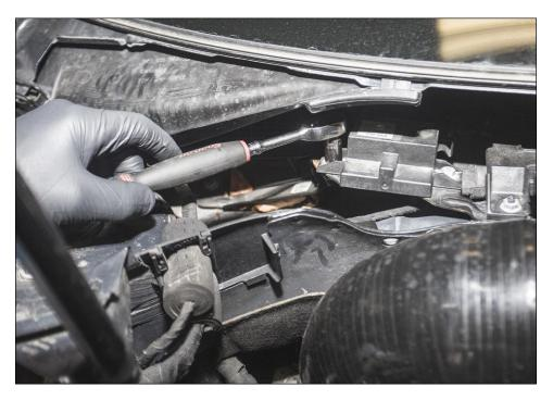
In order to run the wire harness and vacuum lines to the solenoid, the small harness going into the rain tray will need to be modified. To do so, start by carefully releasing the plastic cover securing it. There are two tabs, one on each side that must be released with a small screwdriver.
