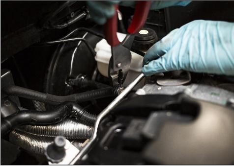
Remove the 5mm triple square bolt from hard line mount tab.
