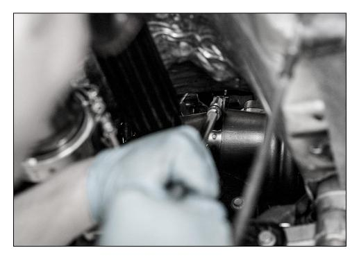
Pry engine forward from the bottom again and slide driveshaft onto alignment pin on the transfer case. Reinstall the three mount bolts, one at a time. Torque each bolt to 60 ft/lbs. This step can easily be performed with the car in gear and the emergency brake engaged.
