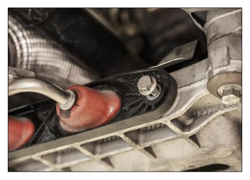
Remove downpipe from car. This step may take some adjusting of the driveshaft and engine to make room for the downpipe on the way out. Once downpipe is removed from car, carefully pull mount bracket from pins. Silicone spray or WD-40 will make this task much simpler.
