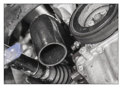
Attach turbo outlet pipe to oil pan using included bolts and washers. You will need a 5mm allen socket for this step.
