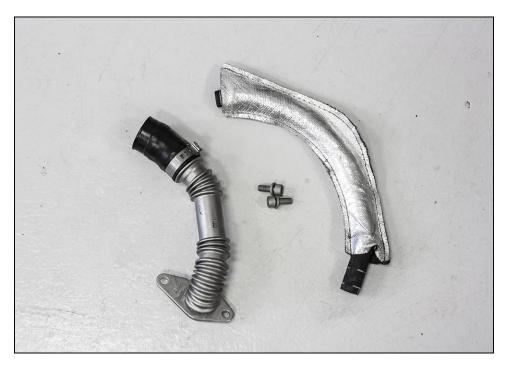
Remove turbo support bracket from block. There are two allen bolts with 6mm heads securing it.
