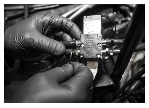
Secure solenoid using the bolt that was previously removed in the rain tray.
