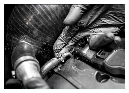
Remove MAF sensor from factory airbox with T20 Torx socket. Using provided bolts, install MAF sensor into IE MAF housing with 2.5mm allen socket. Plug in MAF.
