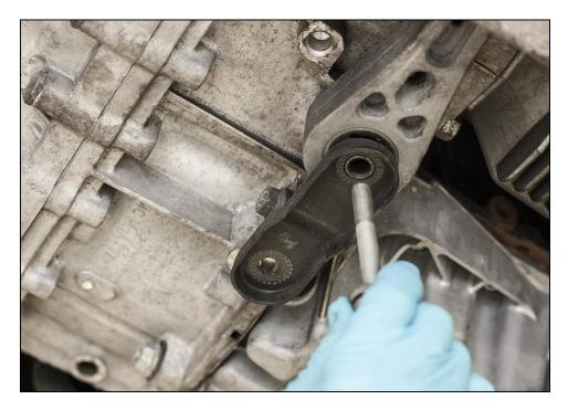
Using a 12-point 10mm socket, remove the three bolts holding the driveshaft to the transfer case. You will only be able to access one at a time, so rotate driveshaft to access all bolts.
