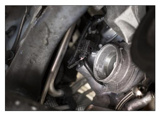
Remove cap screw holding oil feed line bracket to turbocharger using 5mm allen socket.
