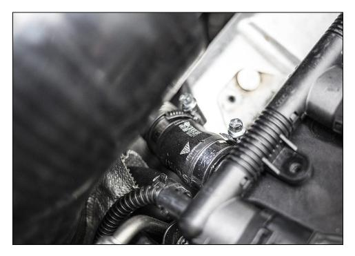
Slide upper clamp onto inlet hose, slide MAF housing into hose. Using included bolts and lock washers, bolt MAF housing to heat shield. Tighten clamp to inlet hose.
