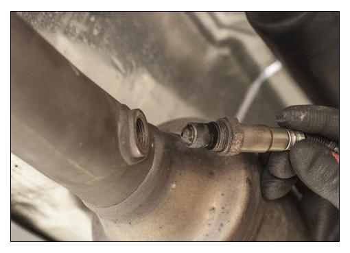
Remove upper oxygen sensor from downpipe and put aside as well.
