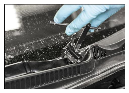
Carefully remove plastic cowl cover below windshield. Once the rubber seal has been taken off the front side, you will be able to unsnap it from the bottom side of the windshield. Start on one side and slowly move towards the other side. Remove cover from car.
