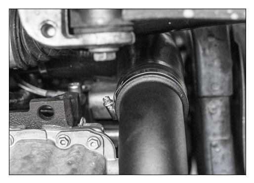
Attach intercooler inlet hose to cast outlet pipe. If using IE FDS intercooler, you will remove the black billet adapter and clamp the hose directly to the cast outlet pipe.
