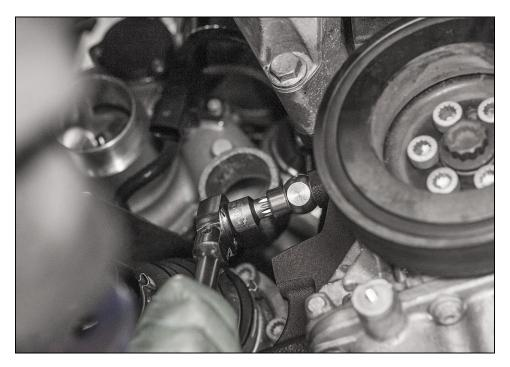
Confirm that oil line is routed properly and not interfering with turbo, manifold, or block. Tighten both ends of feed line with 14mm wrench.
