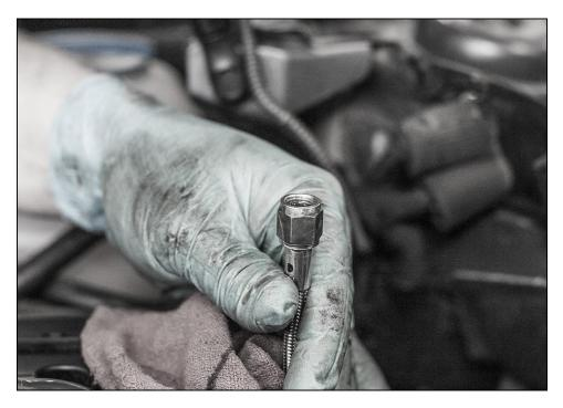
Route oil feed line over turbo, underneath coolant drain line. Install block side of oil line onto the banjo fitting, hand tighten only.
