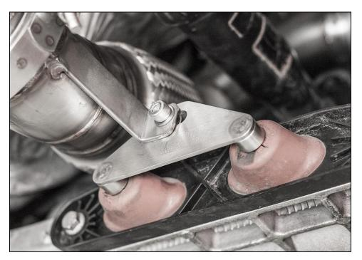
Tighten upper v band clamp, then tighten lower v band clamp. Do not overtighten.
