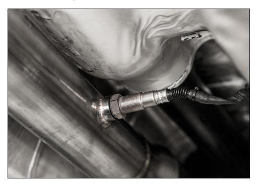
Using same method as above, install oxygen sensor into downpipe.
