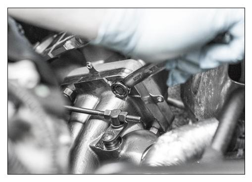
Install new exhaust manifold gasket onto head. Confirm orientation, making sure it is installed correctly. Lightly wipe studs in cylinder head with anti seize lubricant.
