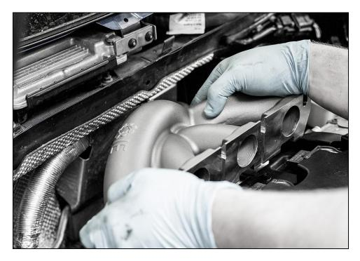
Install nuts onto studs. It is necessary to install the nut on the rear driver side first before starting the other three. Once all four are on the studs, evenly tighten them in a crossing pattern using a 14mm wrench.
