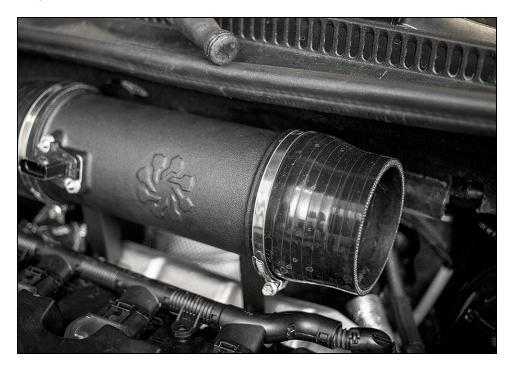
Install aluminum intake tube between MAF housing and velocity stack. Tighten clamps.
