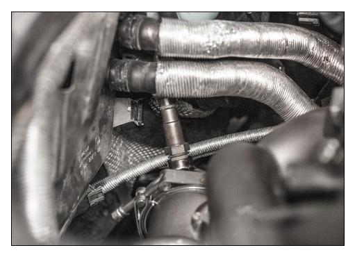
Attach coolant hard lines to turbo heat shield using two 10mm nuts that were previously removed. Reinstall heatshield onto cylinder head using the top two bolts with 13mm heads. The other two original bolts with 18mm heads are no longer used. Ensure that coilpack harness is on the left side of the rear nipple on the hard line.
