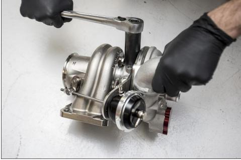
Install coolant drain line on front of turbo. You will reuse the banjo bolt from the OEM turbocharger, along with the two included crush washers (one on either side of banjo) to secure it. Ensure that there is clearance between the coolant line and the compressor housing.
