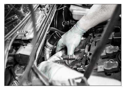
Remove exhaust manifold gasket from head.
