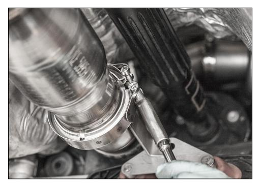
Tighten clamp on rear of midpipe to secure to catback portion of exhaust.
