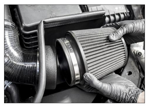
Install step-down coupler onto velocity stack with 80-100mm clamp, do not tighten yet. Slide second 80-100mm clamp onto coupler.
