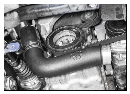
Tighten both hose clamps on turbo outlet coupler. Do not over tighten clamps.
