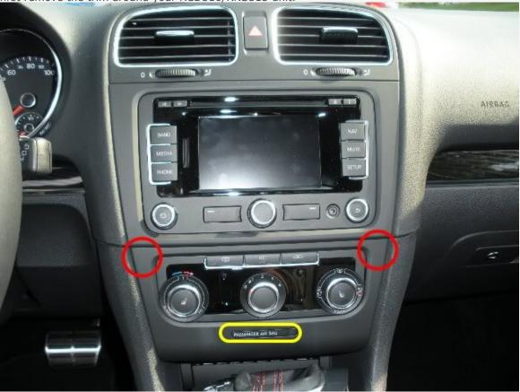
15. Using your trim tool remove the trim around the nav unit by starting from the sides and working your way around.
