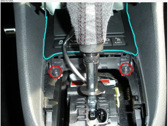
11. Carefully lift up the ash tray and find two wiring harnesses. Remove the white connector (ESP) and the power outlet harness. Note that the wiring bundle for the white ESP connector is attached to a quide (red arrow) which cannot be seen in the photo below. This is easily removed by pulling out to the right (not down).
