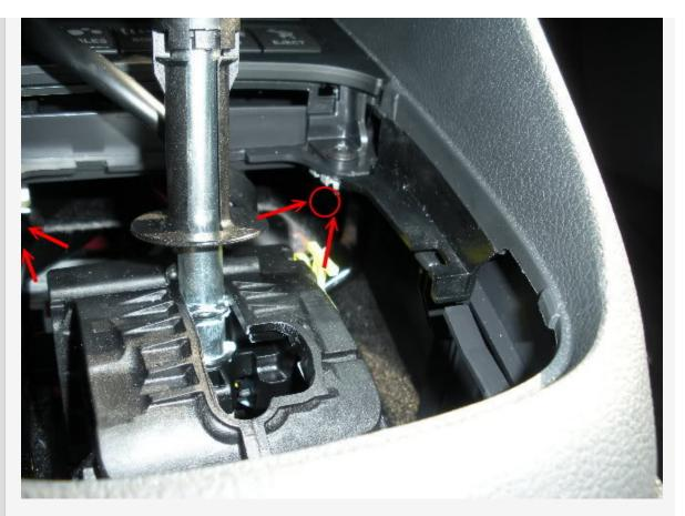
Note: There are two more screws holding the soft trim which surrounds the gear shifter. These screws are located behind the Climate Control trim. To remove the climate control trim you must first remove the trim around your RCD510/RNS315 unit.
