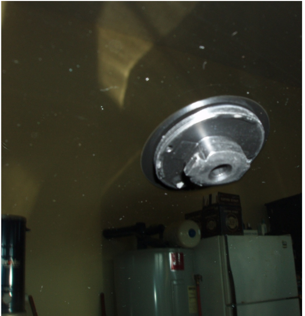
This is what you will mount the new mirror to using the VW adaptor. I painted the horseshoe shaped piece black:
