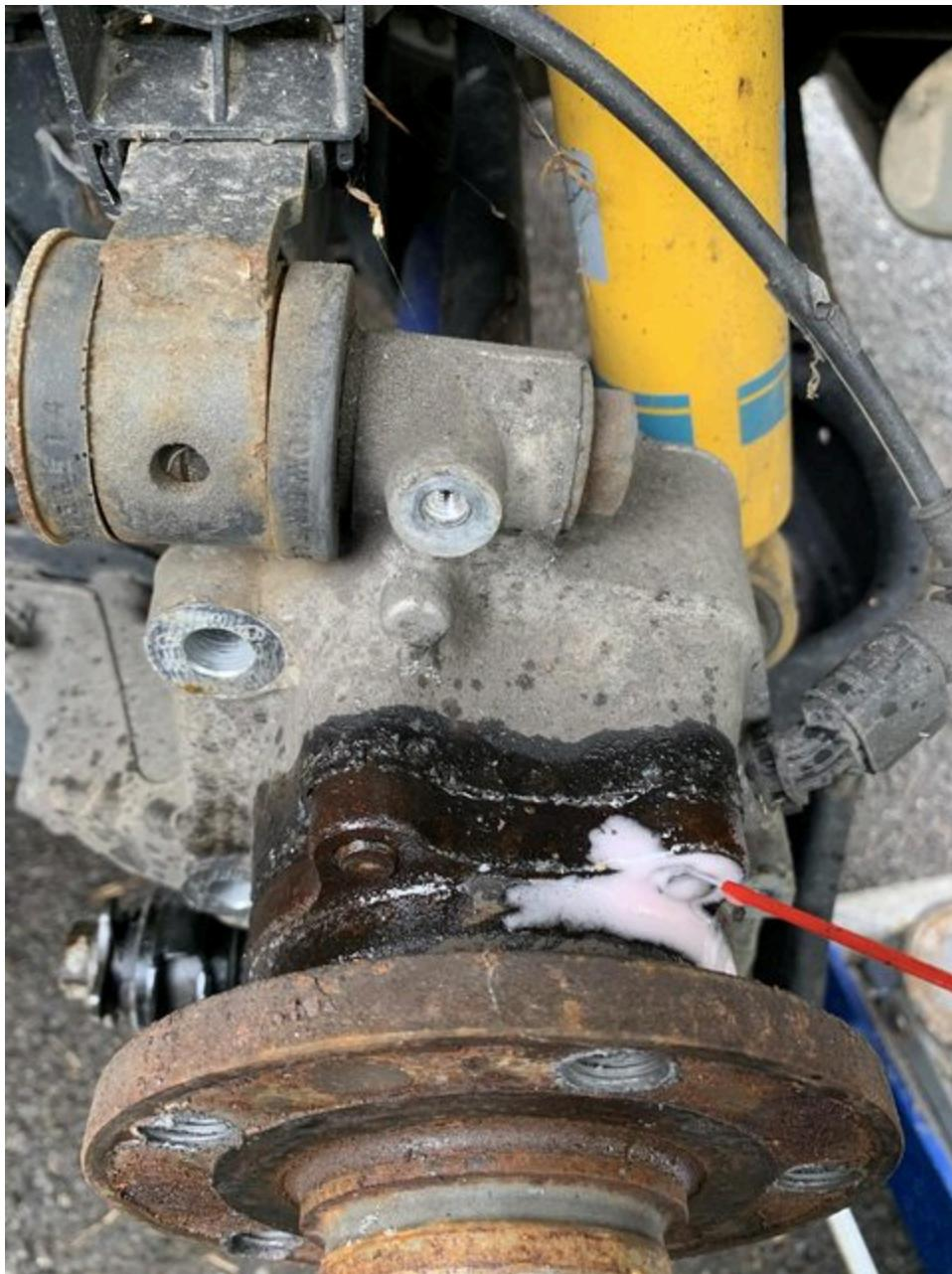
On the back side of the knuckle, you'll see the heads of the mounting bolts for the hub around the CV joint; remove them using the 12mm triple square socket. The hub will likely be stuck to the knuckle with years of grime and corrosion, so you'll need to employ your hammer and prybar to get it off.
