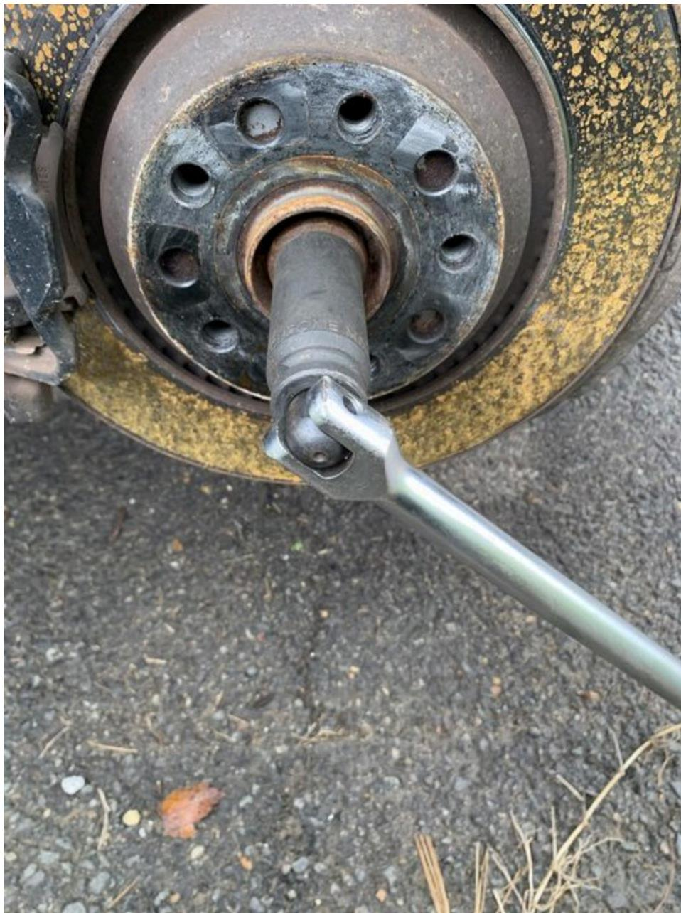
Release the parking brake and remove the brake caliper using the 13mm and 15mm wrenches; tie it off out of the way so that it's not hanging by the brake hose. Remove the caliper mounting bracket bolts using the 14mm triple square socket and set the bracket aside.
