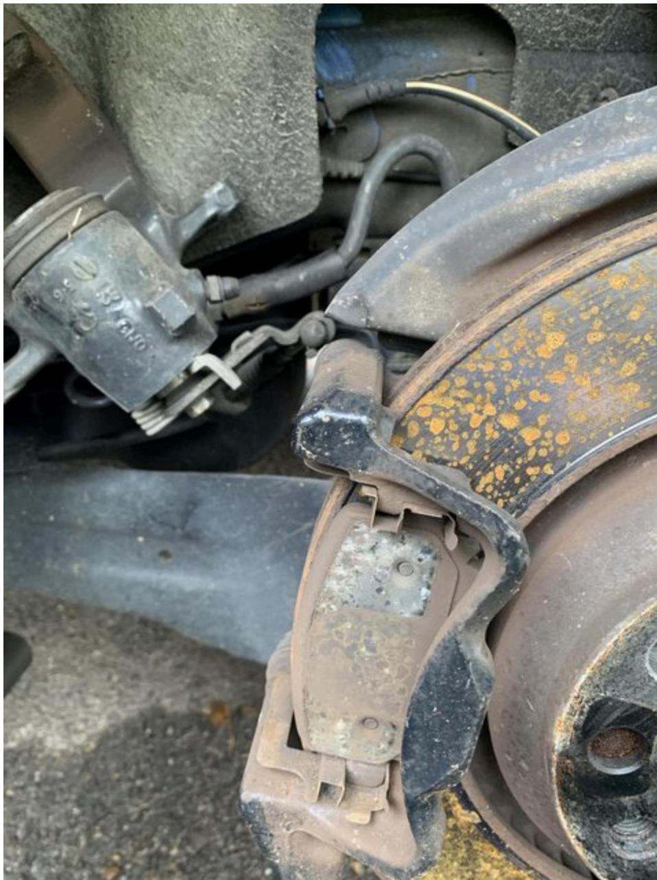
Remove the rotor set screw using the T30 and remove the rotor. You can tap the rotor with a hammer to dislodge it if it doesn't come off the hub easily. Remove the dust shield using the T30. This step isn't absolutely necessary, but it makes access to the back side of the hub a lot easier.
