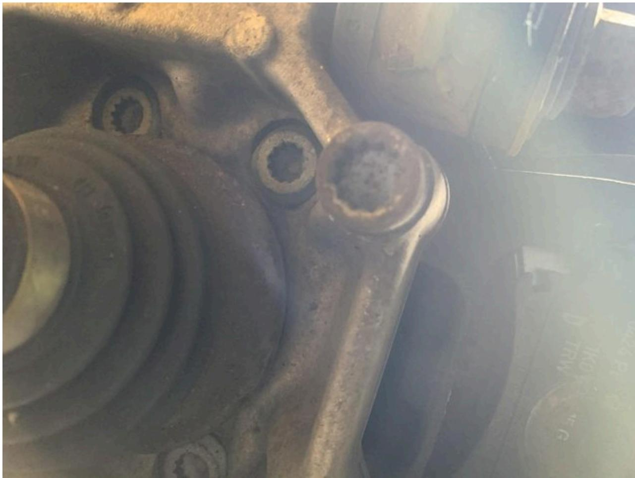
Clean up the mounting recess with some emery cloth, clean and grease the splines on the axle, push the new bolts through the back side of the knuckle, then slide the new hub in place. Make sure the bolt holes are lined up and tap it in place with the hammer, using a block of wood to protect the new hub and even out the Force. You can also use the bolts to draw it up tight, just work in a crisscross pattern (e.g., top left to
