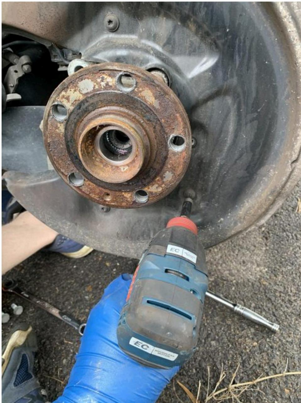
Support the lower control arm at the hub with your jack, and remove the mounting bolt using the 18mm wrench and socket. Let the arm down slowly and remove the spring.
