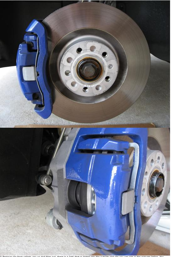
3) Remove clip from caliper, pry up and then out, there is a 'tab' that is sloted into the outside pad clip you can see in the pictures below. You need to pry the clip up till the 'tab' clears the pad clip slot before you can get it outwards towards you. This clip is going to come off with some force, and it very well will scuff off a small portion of the caliper paint.
