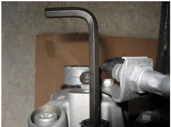
5) Upon removal of the 2 caliper guide bolts, the caliper will slide out and away from the brake disc and you can then remove both inner and outer pads. Remember to have someting to hold the caliper while its off the carrier, do not let it hang on the brake line.
