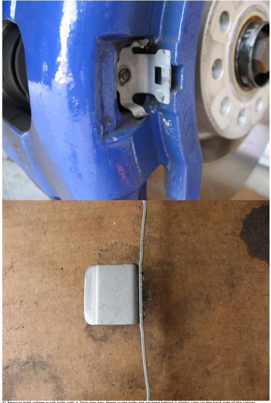
4) Remove both caliper guide bolts with a 7mm hex key, these guide bolts are covered behind 2 plastic caps on the back side of the caliper.
