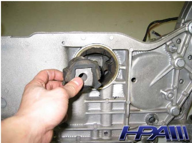
5. Remove plastic outer ring of lower OE mount with channel lock pliers
