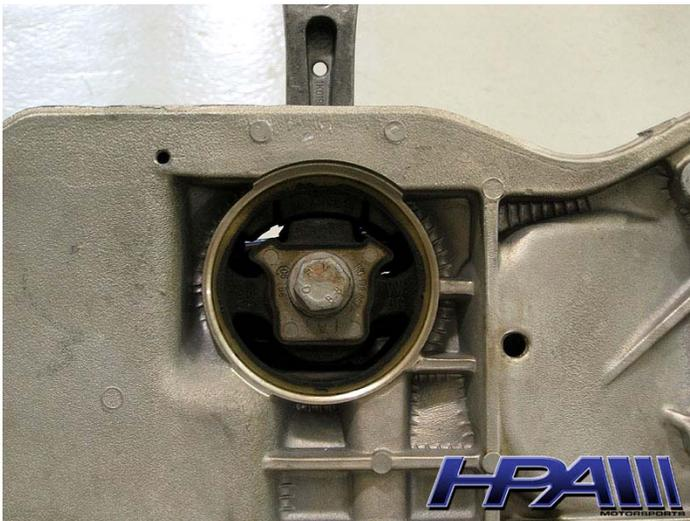
3. Use sharp knife or utility scissors to cut away rubber portion of lower OE Mount
