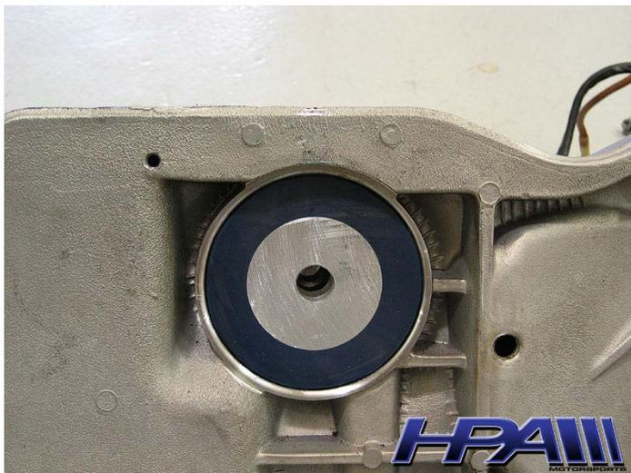
6. Secure core interlock mount with OE bolt. Torque to 50nm plus an additional ¼ turn
