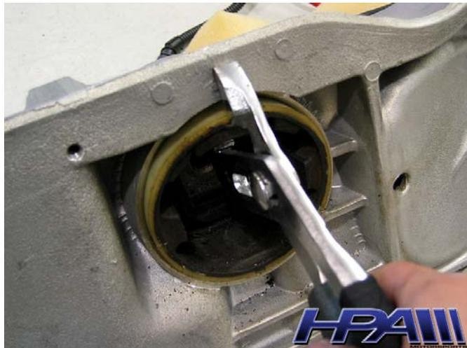
6. Use dish soap to lubricate core interlock mount and install in to sub frame making sure the recess in the mount matches up with the corresponding existing pendulum rod
