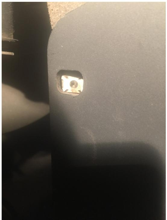
Mark the hole from the stock clip for drilling and then use their provided washer, and the factory screw to secure the third hole.
