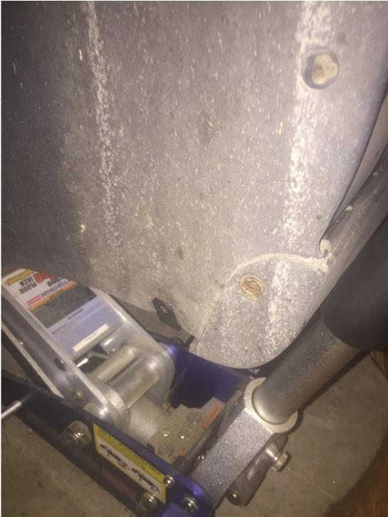
Install provided plastic clip on the bottom of the wheel well.
