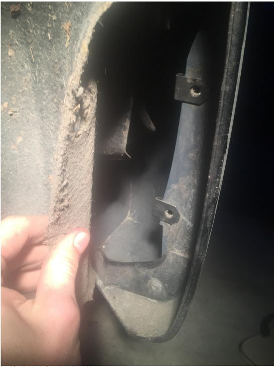
Install Provided plastic clips back into the stock location.
