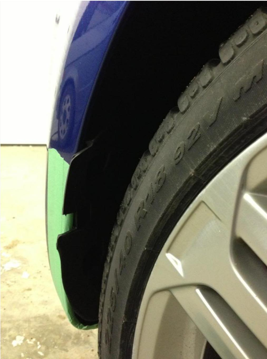
Trace a line where the lip of the core passes over the fender, this will need to be trimmed also.
