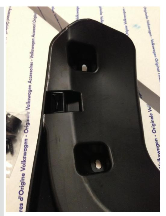
I find you don't need to cut all the way through the first pass, as the outer textured shell can actually be pulled away from the core if there is a guide cut.
