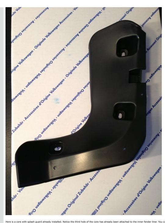
Here is a core with splash guard already installed. Notice the third hole of the core has already been attached to the inner fender liner. You can use an awl or a drill to puncture a guide hole in the fender liner, then use one of the Torx20 screws and a nylon 10mm nut to secure the backside of the liner.
