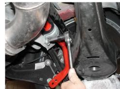
Install NEUSPEED anti-roll bar using original clamps and bolts to sub-frame. Torque bolts to 20Nm (15 ft-lbs).
