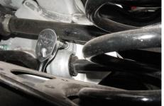
Remove four bushing clamp mounting bolts using a M10 Triple Square or 8mm hex key wrench. Now remove original anti-roll bar from vehicle. NOTE: To access upper clamp bolts, suspension must be compressed to raise drive axel.
