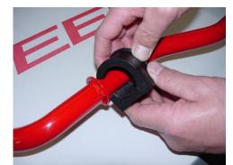
Apply silicone grease to the inside of supplied bushings and install on the inside of stop washer on NEUSPEED anti-roll bar.
