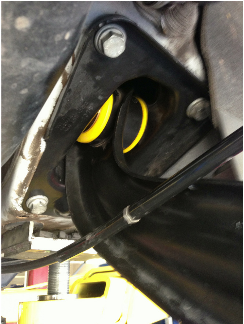
#5 - 2x18mm Bolts - 66ft/lbs + additional 45 degrees
