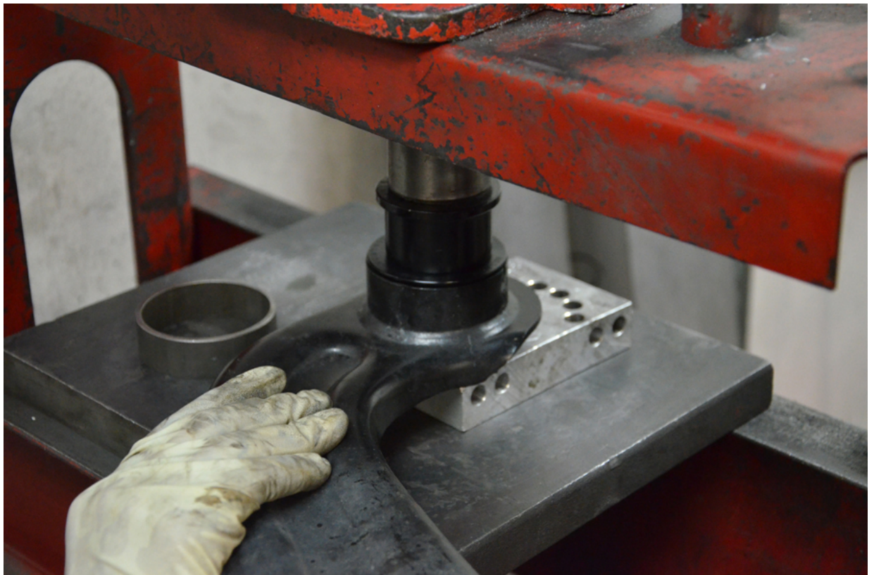
Step 14 – Reinstall spacers into spherical trailing arm bearing.
