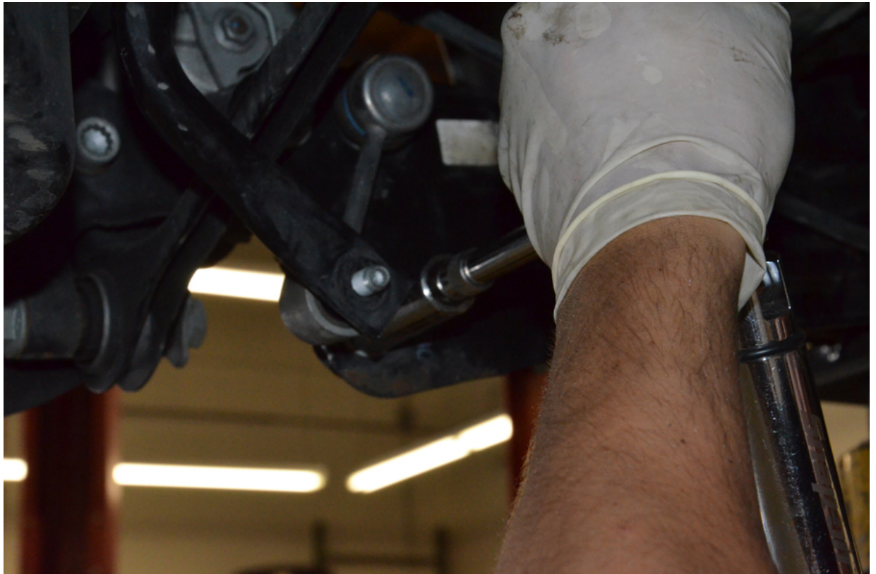
Step 19 – Reinstall parking brake cable retaining clip with T30 screw torqued to 8Nm.
