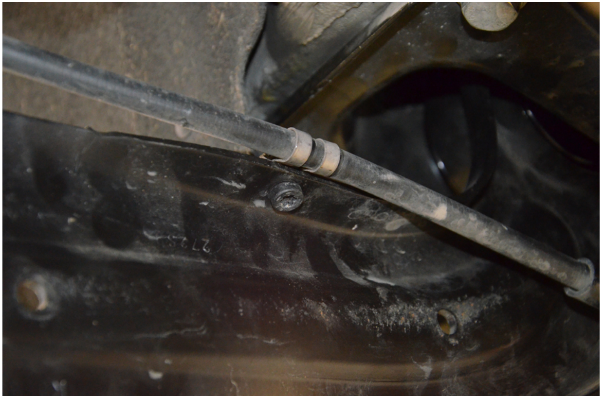
Step 20 – Reinstall end links. Torque end link hardware to 45 Nm.
