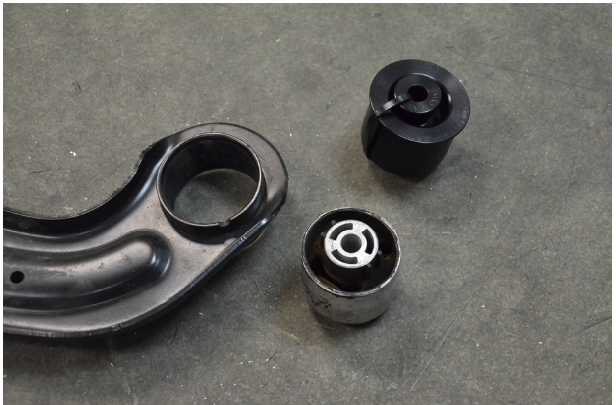
Step 11 – Clean up the inside bore of the trailing arm using supplied sanding drum.
