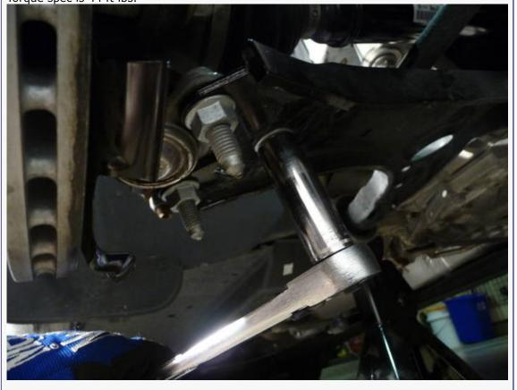
Have a friend hold the brake while you install a new drive axle bolt. VW part number WHT-002-795.
