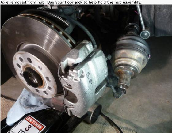
Remove the strut lower bolt/nut
