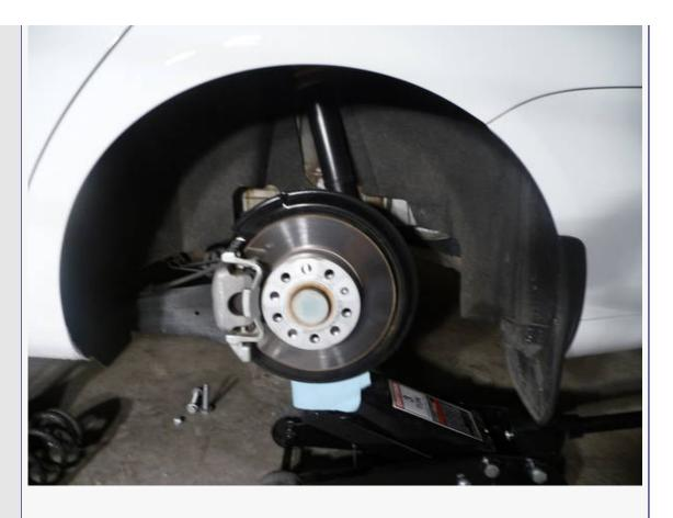
Transfer the upper rubber mount pad to new spring. Install the sport spring, ensure bottom end of spring is butted against the stop molded into the rear lower control arm. Raise the rear lower control arm back up using the floor jack. Install new bolt and nut. VW part number. Bolt = N-106-286-01, Nut = N-101-064-02. Torque spec is 66 ft lbs + 90 degrees.
