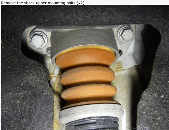
Pry the plastic cover off the rear shock to allow access to the upper nut, remove this nut.
