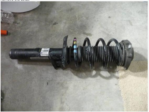
Compress the spring with spring compressors. I got mine from autozone loan-a-tool program.
