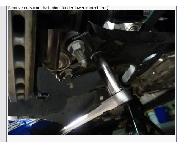
Push down on the lower control arm to remove it from the front hub. Pull outer joint of drive axle out of wheel hub. My car only had 5300 miles on it but my drive axle would not come out of the hub. I had to get a hub puller and push it out. It came right out with the puller. I went to Oreillys and used the Evertough 67032 front wheel drive hub puller from their loan-a-tool program. I had to use a long socket to give the puller screw enough length to completely remove the axle out of the hub.
