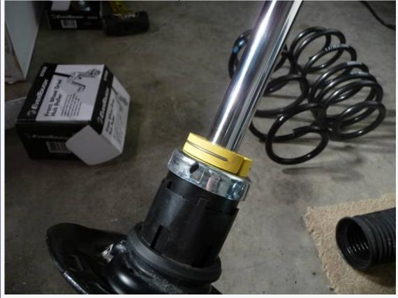
Reassemble the strut with the new spring. Ensure the bottom spring end is butted up
