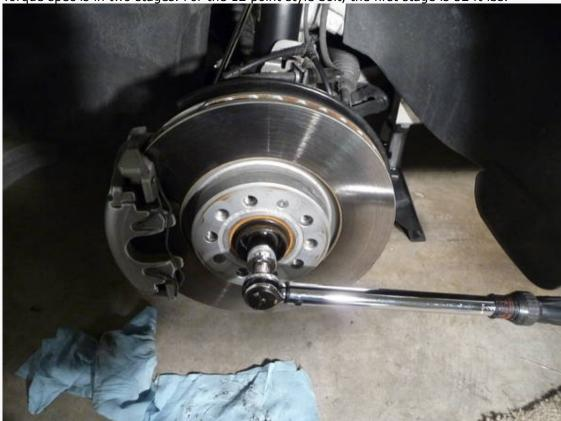
After torquing to 52 ft lbs, install the wheel with the center cap removed. Put the vehicle weight on the wheel and tighten the drive axle bolt an additional 90 degrees (second torque stage). You will need a long breaker bar for this. I used a 24mm 12 point socket with a 2 foot breaker bar to get the 90 degrees.
