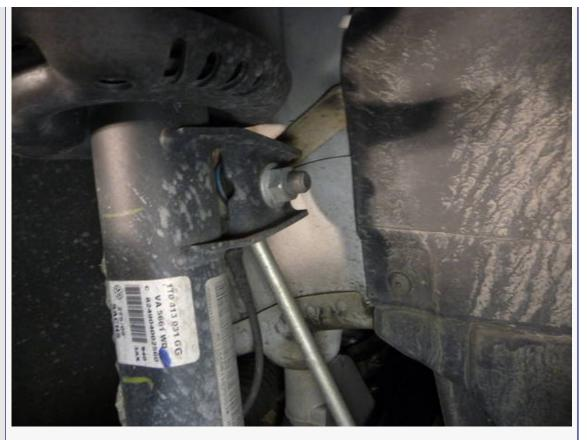
Install new nuts for the lower control arm to ball joint VW part number N-103-320-02. Torque spec is 44 ft lbs.
