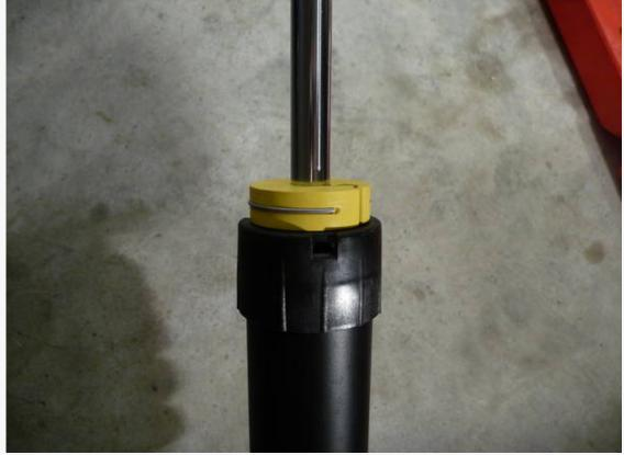
Install shock. Upper bolts first. Torque spec is 37 ft lbs + 45 degrees.
