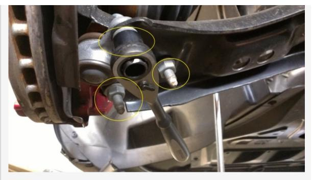
10. Push down on LCA so they come off and away from ball joint, just push it down and out of way best you can,do both sides of car.
