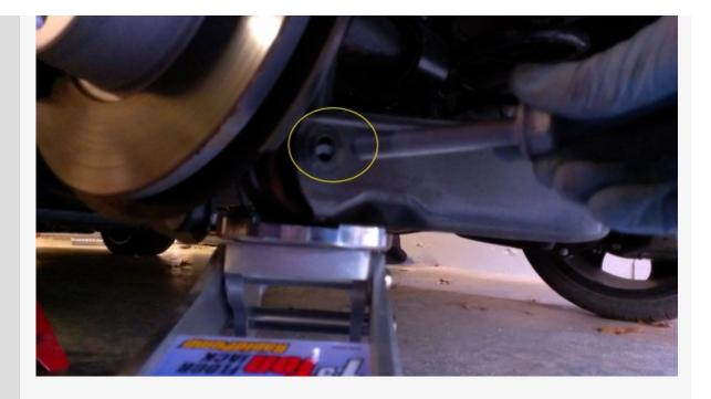
14. Install 18mm nut and torque down.
