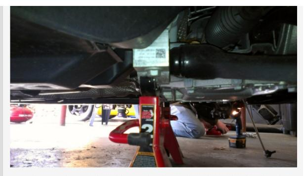
5. now that one side is on jackstand, lower jack and go to other side, it makes the job much easier and faster to get entire front up in air.
