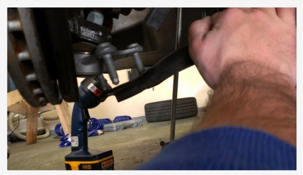
11. PINCH SPINDLE: At bottom of strut, using a M14 Triple Square on stretch bolt, and 18mm deepwell socket on nut, remove the stretch bolts that "pinch" the spindle around strut bottom. at this time do one side of car( as you can see i didnt have a M14 bit, i used a 3/8 extension to hold and torqued the other side).
