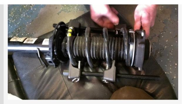
18. once compressed, remove the large 21mm NUT on top of strut. This is where a special tool is needed, I ended up buying a offset box wrench set at harbour freight for only \$15 for entire set, they did not have a set with 21mm though, so i got SAE set and used the 13/16 size which worked perfectly. You need to hold the middle shaft with 7mm allen wrench/socket. Notice Tape on rearward hole.
