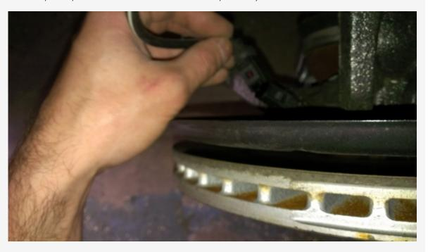
8. Locate the sway bar link, and remove the top 18mm nut that attaches link to strut, Just lay each link down out of the way. Do BOTH sides of car.
