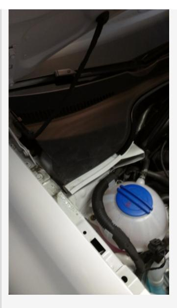
16. Loosen the 13mm bolts, on the last bolt reach down and hold the strut with one hand so it does not drop when you remove last bolt. As you pull out strut, make note of the REARWARD hole, take some blue tape and put a piece of tape around edge at the rearward hole. this will assure the strut mount/bearing plate goes back in exactly then same later.
