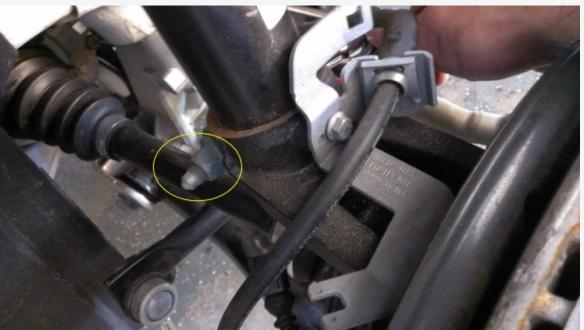
12. Using a strut spreader tool, insert tool into rear slot, and twist it 1/4 turn to open the "pinch" on spindle (i didnt have a strut spreader, tried a 1/4 inch extender).
