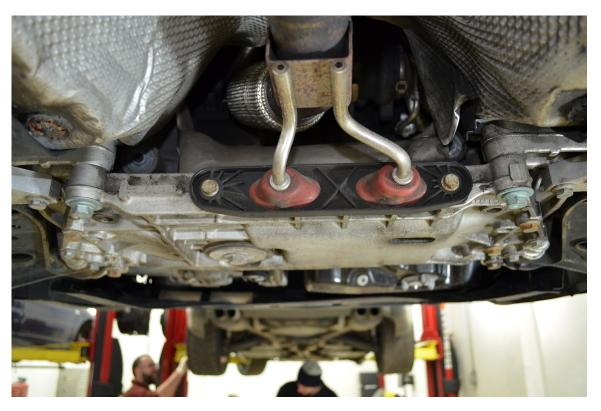
Next is to remove the two bolts from the dog-bone mount to the transmission. This is done with a 16mm socket.
