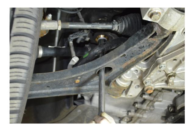
Tighten the bolts with the collars by hand until they sit flush.
