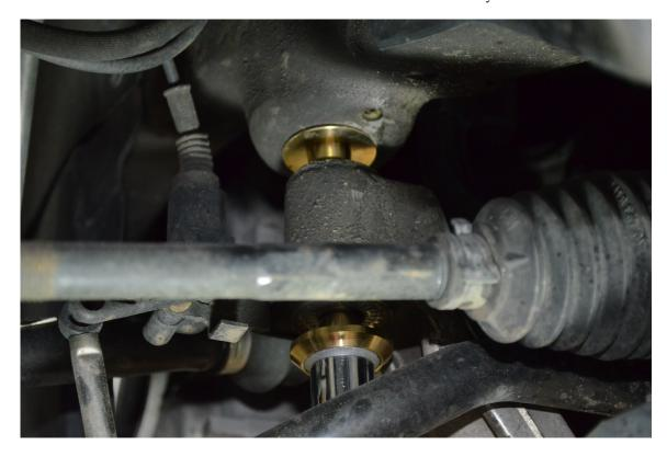
Above, the socket shown on the upper sub-frame bolt to assist in hand installing of the bolt since this one is difficult to reach. The upper sub-frame mount will receive the collar with the large diameter recess for the factory larger shoulder bolt.
