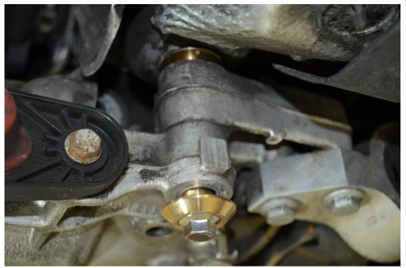
Install all of the bolts one at a time with the collars and let the sub-frame hang. By installing every bolt collar one at a time it keeps the sub-frame from shifting too much. Each side (passenger & driver side) will receive three collars and 3 wedges.
