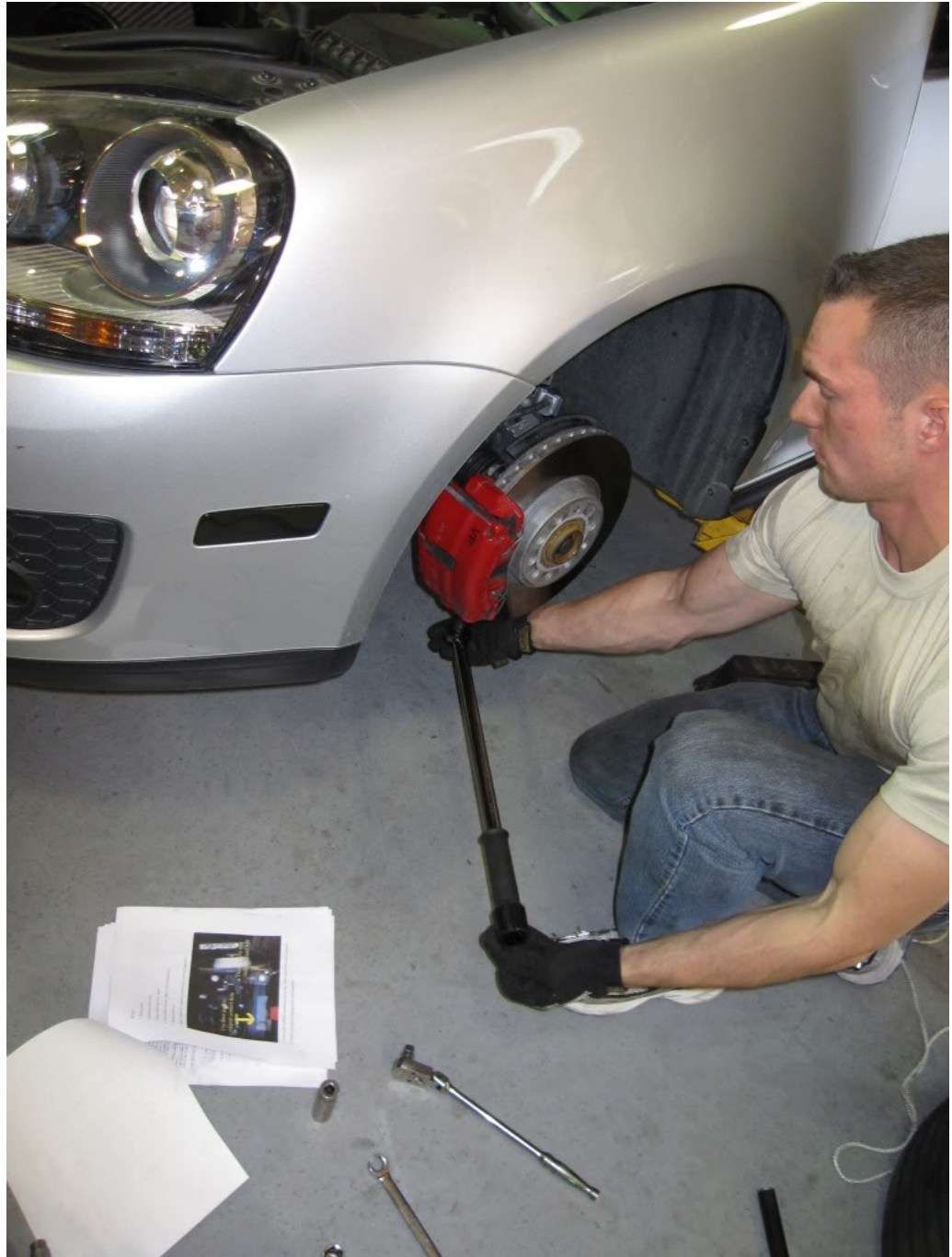
28. Install M14 pinch bolt and 18mm nut at bottom of strut/hub. Torque to 70NM+90 degrees.
