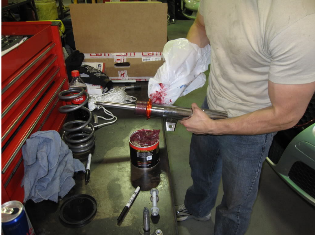
21. Put the white split washer on the strut followed by the new bumpstop, and then the dust cover.
