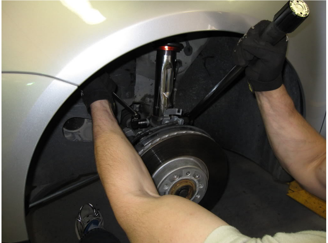
29. Reattach HID leveler arm using 10mm socket and needle nose pliers. The joint in the leveler arm should be pointing towards the driver side.
