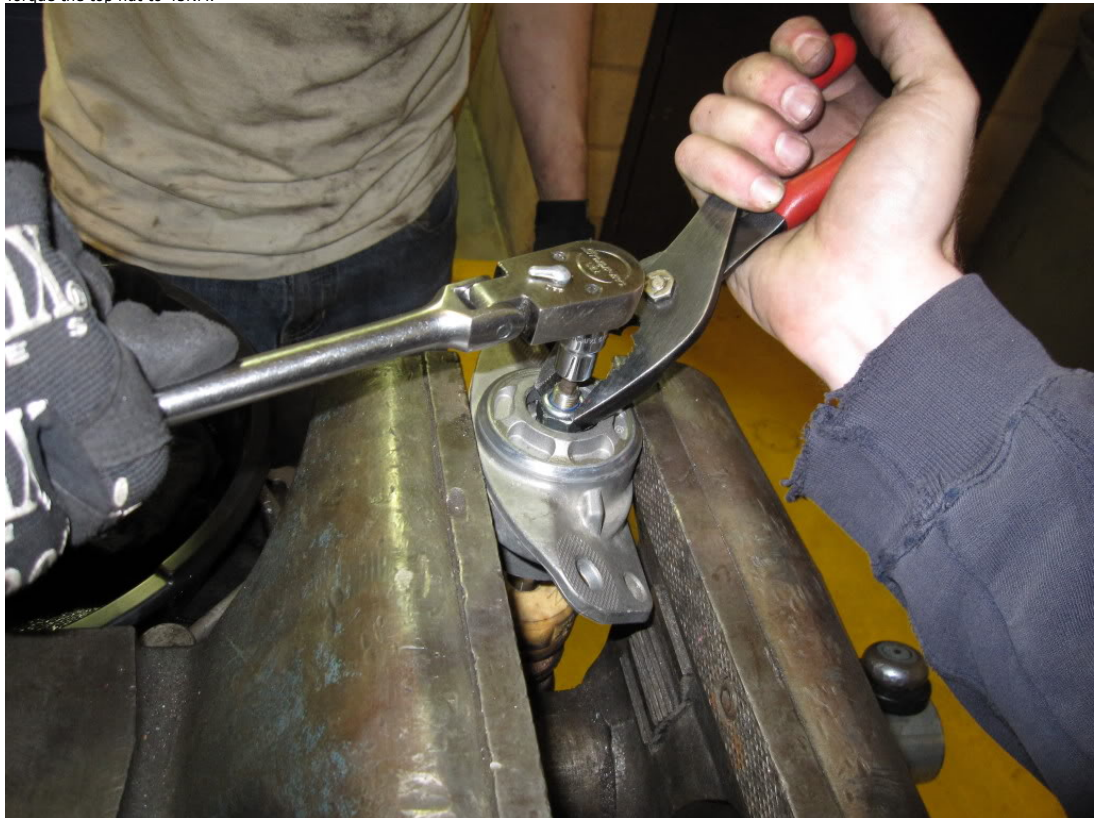
14. Install new rear strut assembly. Tighten 21mm nut. I do not have torque specs for this.
