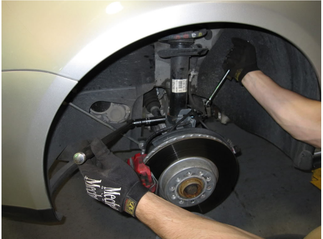
9. Remove the 3 16mm nuts holding the ball joint to the control arm.
