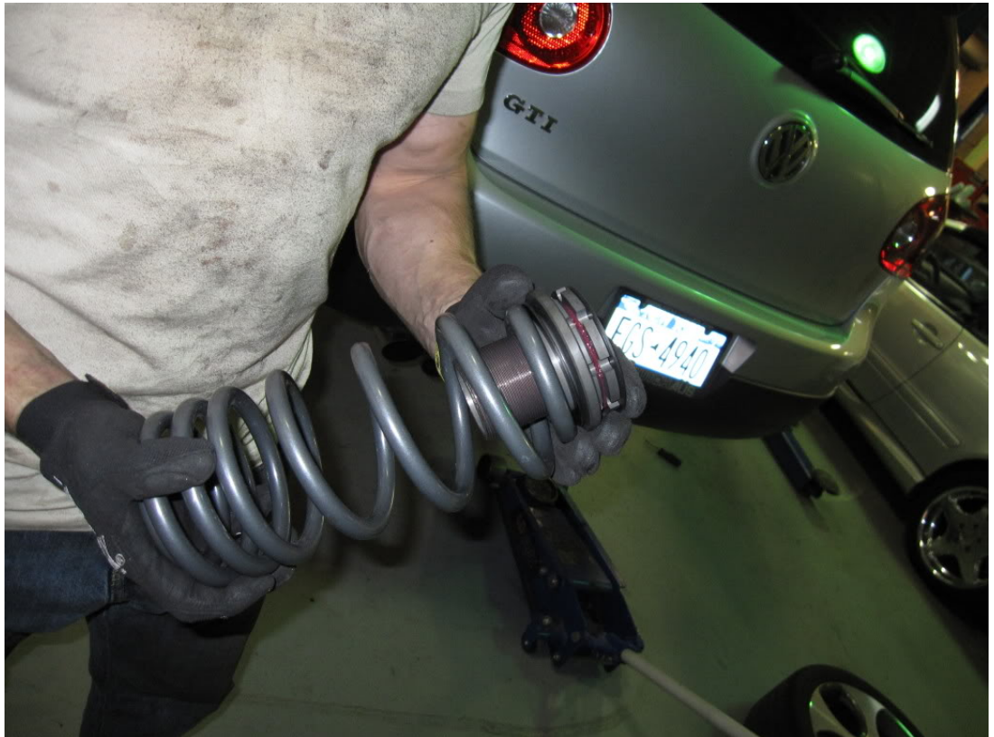
17. Install the new spring. Place into the bottom of the control arm in the same orientation that the stock spring was. The bottom of the spring should look like this in the base of the control arm, so that the end of the spring rests against the nub the arrow is pointing to:
