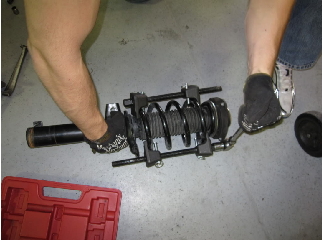
18. Remove the 21 mm nut on top of the stock strut. Use the 21mm side of the specialty tool double sided socket. Then pass a 7mm allen socket on the end of an extension through the double sided socket. This prevents the strut shaft from spinning while removing the 21 mm nut.
