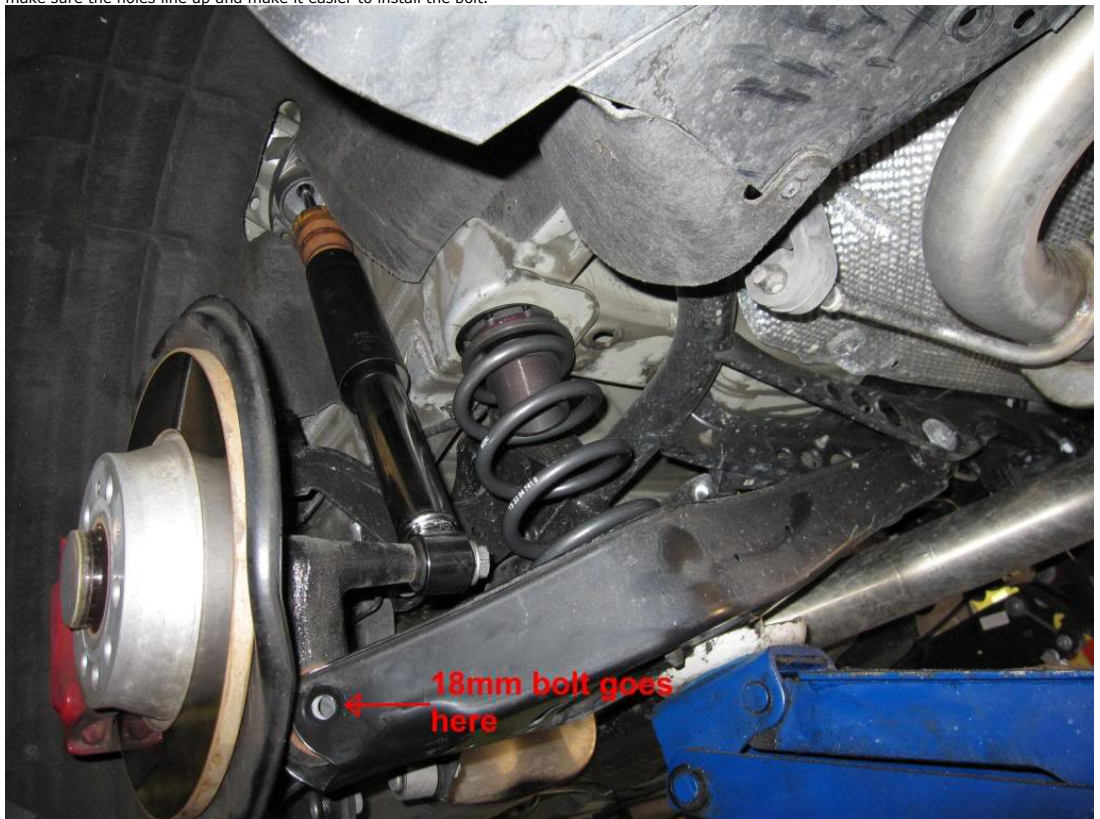
20. Install the 16mm bolts in the strut mount. I do not have torque specs for these.
