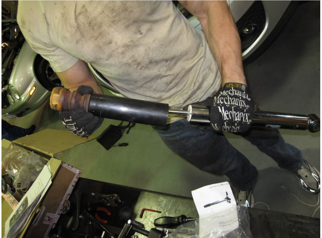
13. Install the new strut assembly into the strut mount. Use the new 17mm nut provided and tighten down on the top of the strut. The tool is a deep socket 17mm box wrench and a 7mm allen socket. I did not have the deep socket wrench so I improvised as you can see in the pictures. Torque the top nut to 45NM.
