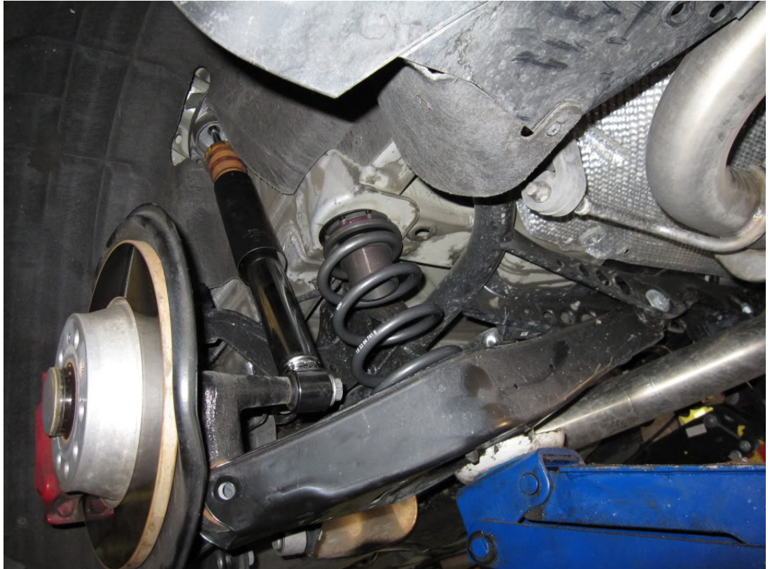
19. Insert the 18mm bolt and 18mm nut connecting the control arm and hub assembly. Tighten to 90NM+90 degrees. Raise and lower the jack to make sure the holes line up and make it easier to install the bolt.
