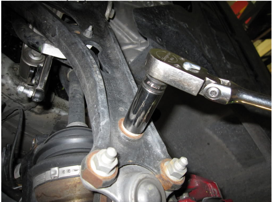
10. Remove the axle bolt. You should have already loosened it at this point.
