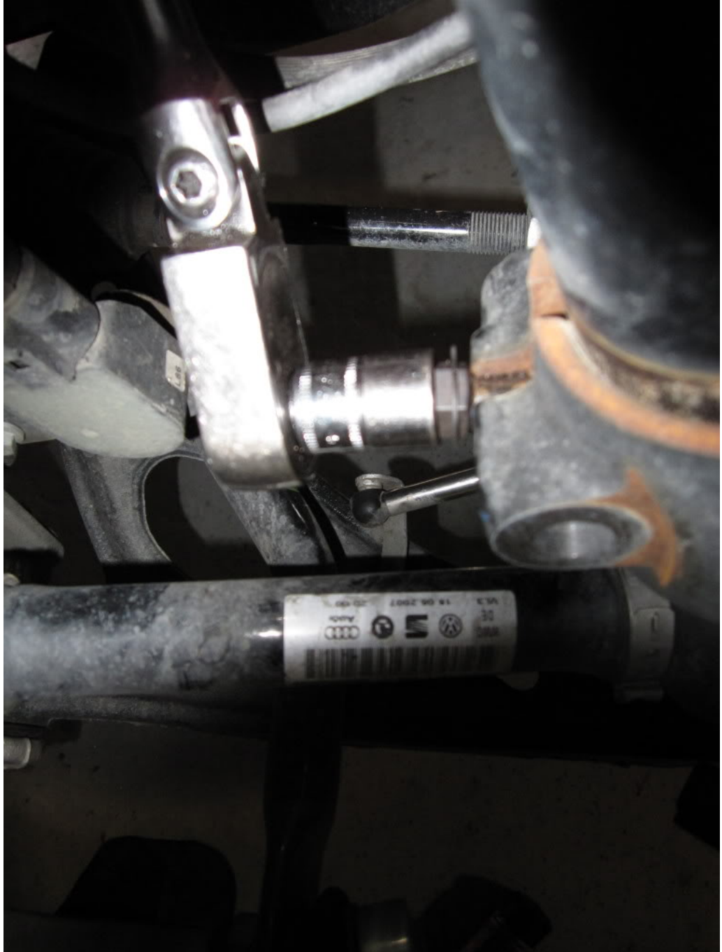
12. Separate the ball joint from the control arm. This will take a little force and maneuvering around. I found it easiest to push down on the control arm while using a flathead screwdriver to pry between the ball joint and the control arm.
