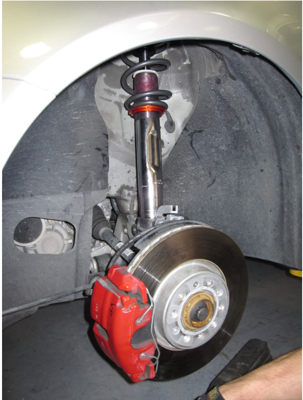
27. Tighten three 16mm ball joint bolts to 60NM.
