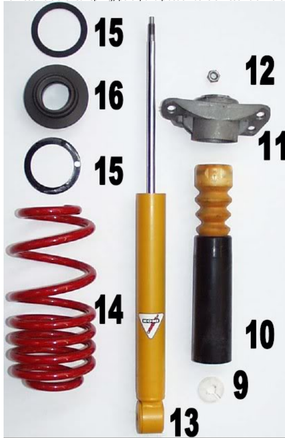
16. Assemble the rear spring, perch, and plastic washers. Assemble in the order shown below. Make sure the spring is in the correct orientation.
