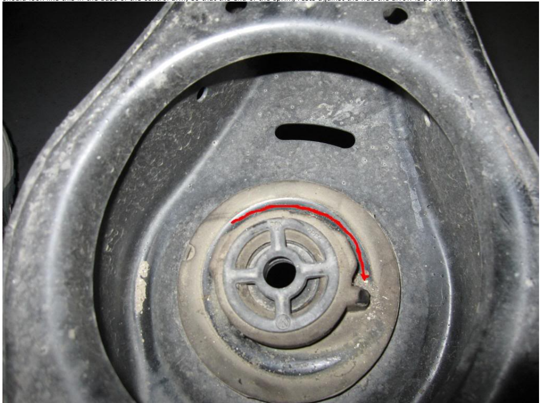
18. Jack up the control arm making sure the top of the spring and perch assembly sits correctly on the nub on the frame of the car.
