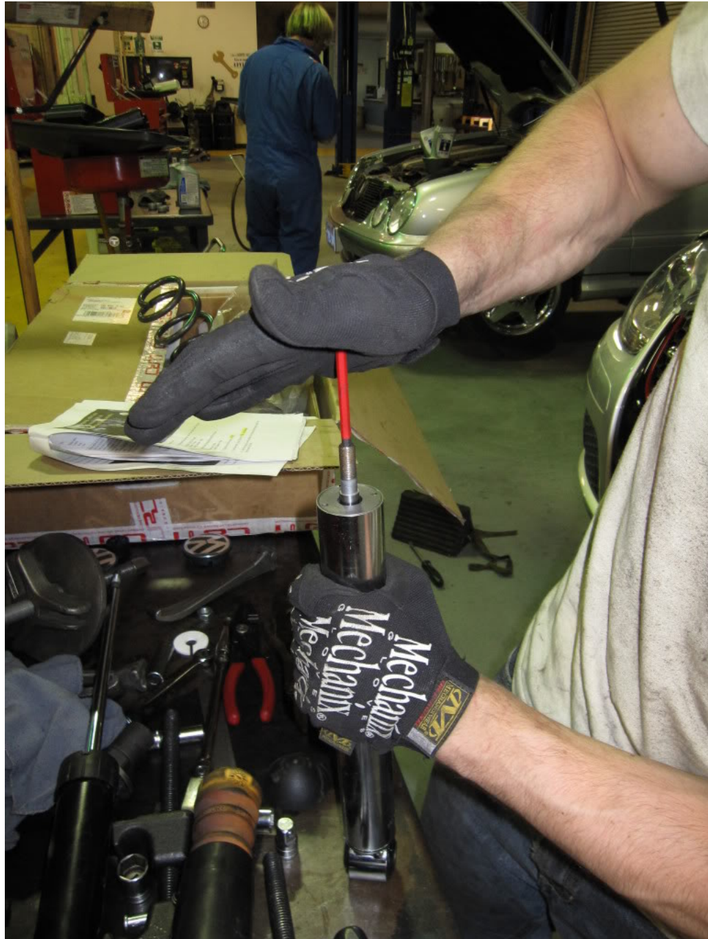
12. Assemble the new strut. First slide on the new white split washer, followed by the bumpstop and dustcover.
