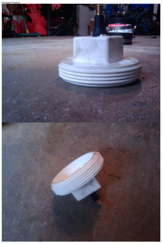
At this point use the epoxy if you like, mine was so tight there is no chance air is leaking out. Just be careful where you apply it, do not fill the valve with glue or air cannot pass through.
