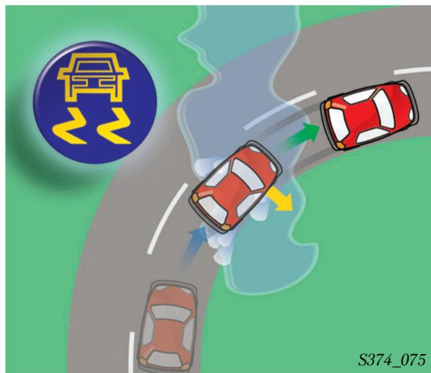
TCS reduces the driving power and therefore prevents excessive slip at the drive wheels. The lateral guidance forces are able to act and the vehicle's driving behaviour remains stable.
