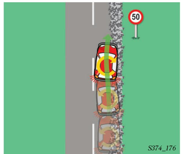
In a vehicle with countersteering support, correspondingly targeted steering forces are applied via the power steering system to support the driver in countersteering. As a result of this, the stopping distance is reduced, there is less deviation from the course and the vehicle's stability is increased.
