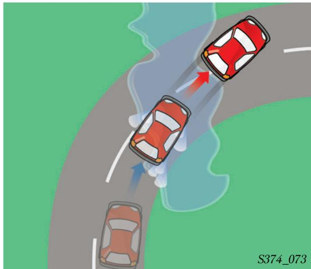
The vehicle accelerates on a slippery road surface. The wheels spin and the vehicle is not accelerated or is only accelerated very slowly. On cornering, only insufficient lateral guidance forces can be transmitted and the vehicle cannot be steered.
