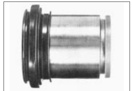
3.9 Dust seal location on caliper piston
