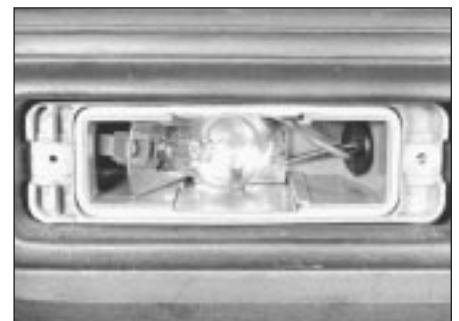
8.5 Front indicator lamp bulb
