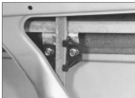
20.3b Lifting plate-to-window channel bolts
