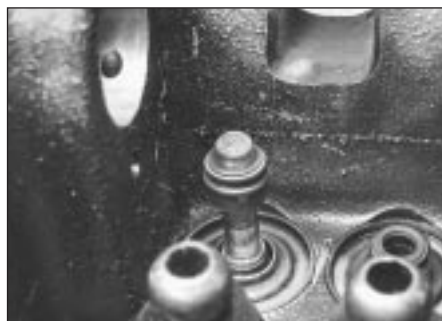
34.4 . . . then fit the new oil seal
