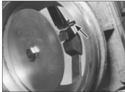
14.6 Airflow sensor plate adjustment clip (arrowed)
