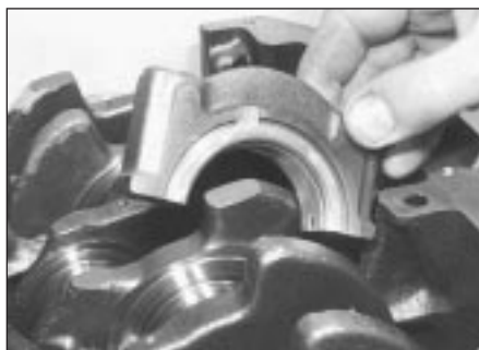
30.5 Fitting main bearing caps
