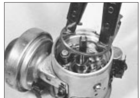
7.10b Removing bearing plate retaining ring
