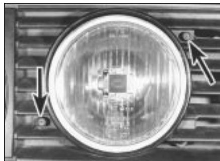
7.4 Foglight beam alignment adjuster screws (arrowed)
