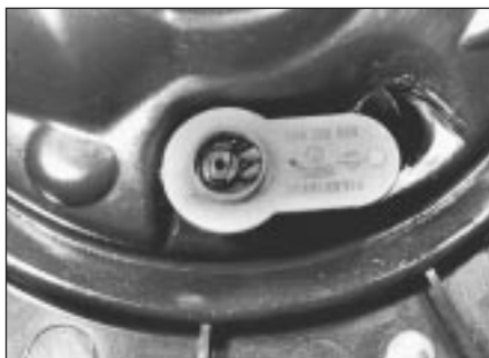
4.5 Upper view of air temperature sensor - 1.3 litre
