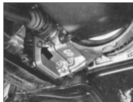
35.10 Final drive unit oil filler/level plug (arrowed)
