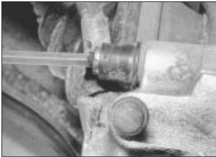
2.3a Caliper securing bolt removal
