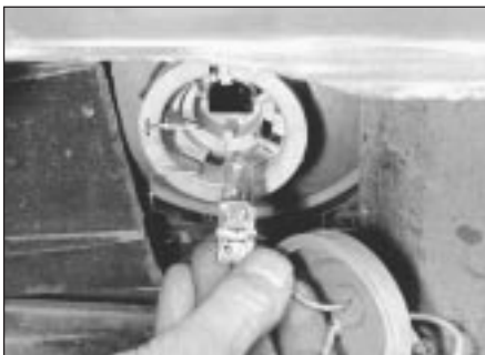
7.2 Bulb and holder removal from foglight
