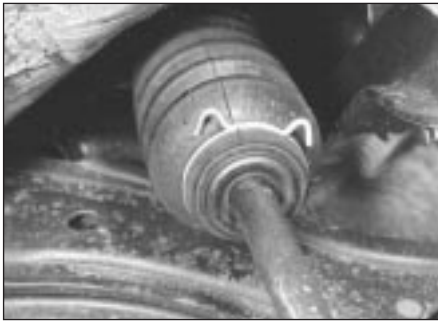
14.4 Steering tie-rod bellows and retaining clip
