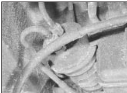
21.1 Fuel accumulator unit location
