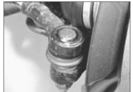
28.2 Inspect balljoint dust covers
