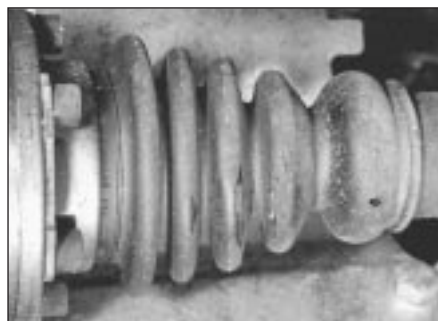
24.2 Inspect condition of each CV joint boot
