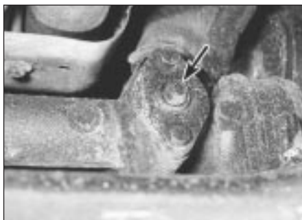
16.1 Manual steering gear adjustment screw (arrowed)
