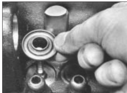
11.4 . . . and valve spring lower seats
