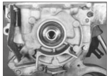
31.4 Fitted location of oil pump
