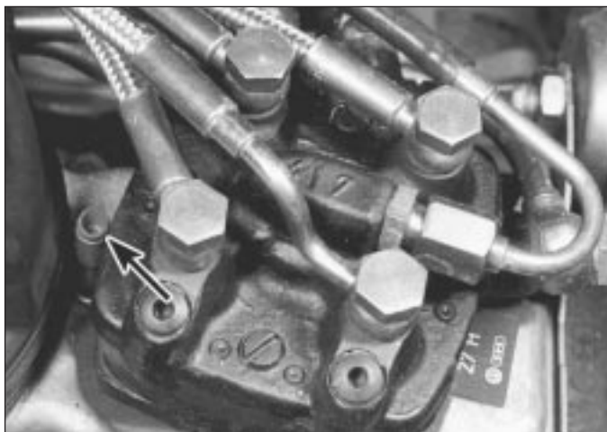
7.2 Idle CO adjustment screw location (arrowed)
