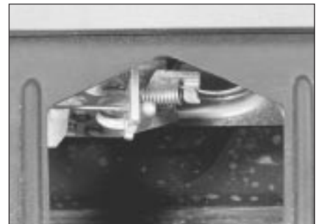
7.4 Bonnet release cable-to-lock attachment
