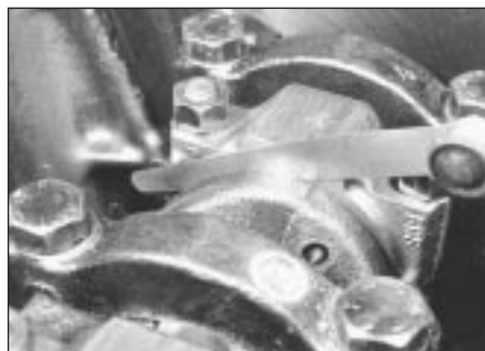
17.4 Checking connecting rod endfloat
