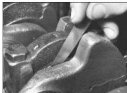
15.3 Checking crankshaft endfloat at No. 3 main bearing
