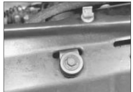
3.5 Radiator central retaining bolt and bracket
