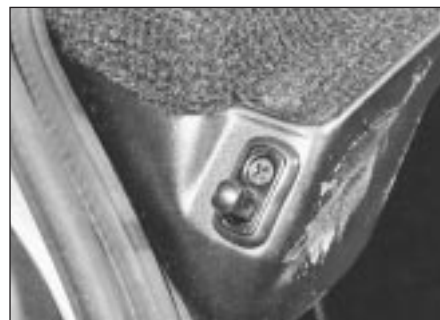
14.2 Tailgate actuated luggage compartment light switch
