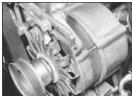
13.4b Alternator drivebelt tensioner link - 1.8 litre
