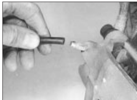
12.5 Connect bleed tube to bleed valve
