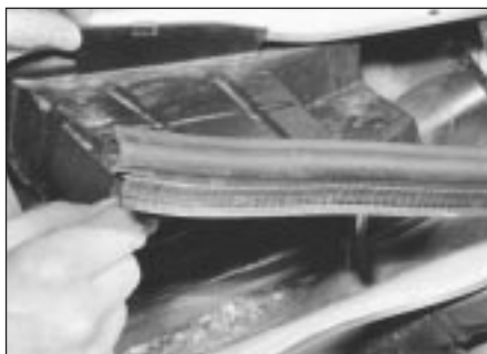
4.2a Carefully prise free plastic cover . . .
