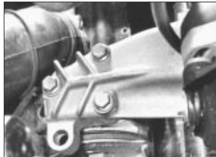
5.24 Engine mounting/bearer - right-hand
