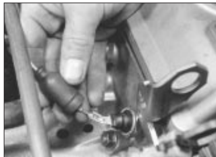
11.23c Oil pressure switch electrical connection
