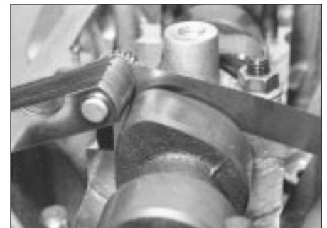
8.6 Measuring camshaft endfloat
