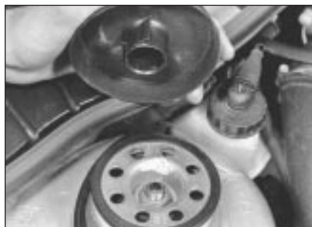
2.3 Removing front suspension strut top cap
