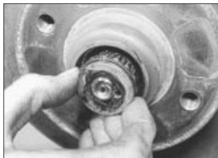
4.15 ... followed by the outer washer and bearing
