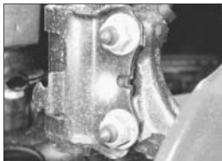
2.7 Strut-to-front wheel bearing housing retaining nuts/bolts
