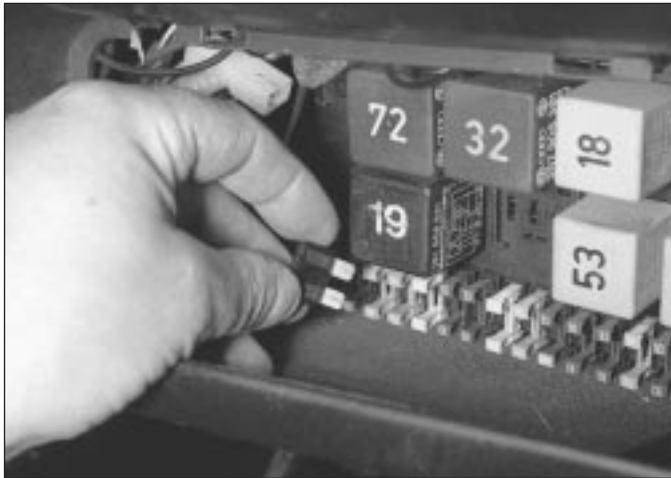
3.2 Removing a fuse
