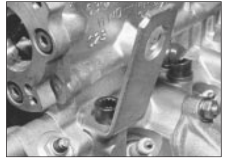
5.23 Engine lifting eye
