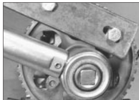
35.5 Method of tightening camshaft sprocket bolt
