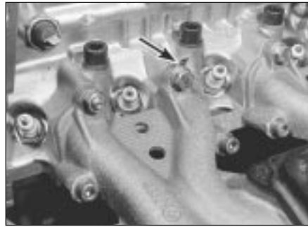
19.6 Inlet manifold-to-cylinder head securing nuts and bolts
