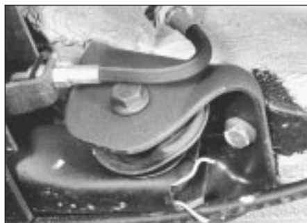
9.7 Axle beam pivot bolt head fitting position
