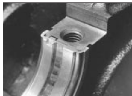
30.3f Ensure that ends of bearing are flush with joint face
