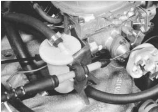
10.3 Accelerator cable to carburettor throttle control
