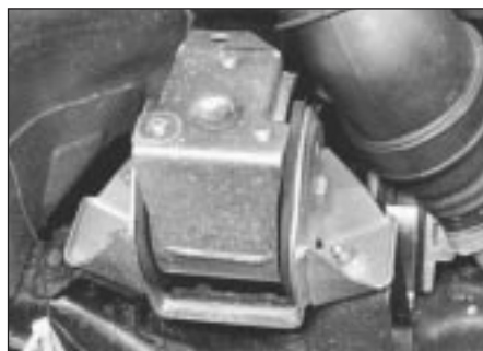
8.1b Right-hand rear mounting viewed from above
