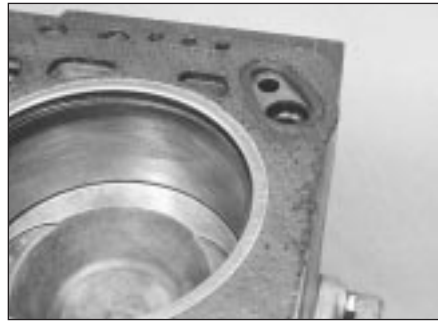
36.2 Correct fitting of cylinder head gasket
