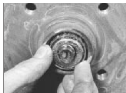
6.5c ... and outer bearing
