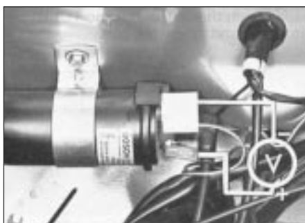
4.6b Voltmeter connection to coil when testing ignition switch unit and coil
