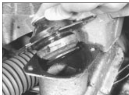
8.1a Lift the mounting away
