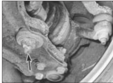
4.2 Anti-roll bar eye bolt nut (arrowed)
