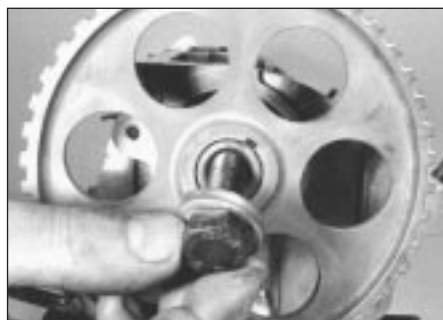
10.10 Removing camshaft sprocket bolt (early type sprocket shown)
