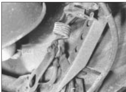
9.3 Brake pressure regulator unit showing spring bracket
