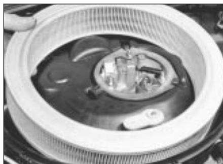
32.2 . . . and remove the element - 1.3 litre, carburettor
