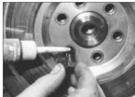
33.3 Applying liquid locking fluid to flywheel bolts
