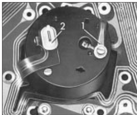
17.4 Normal type clock connections
