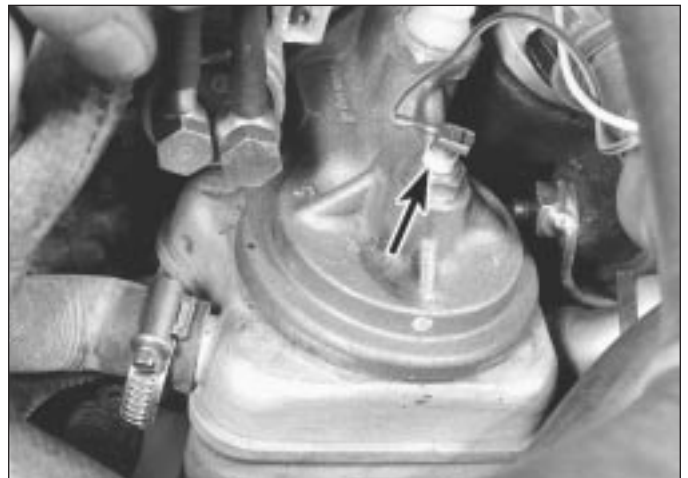
5.39 Oil temperature sender (arrowed)
