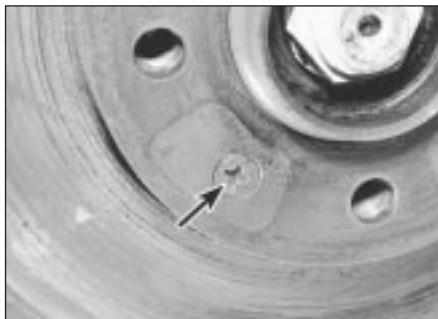
4.5 Front brake disc retaining screw (arrowed)
