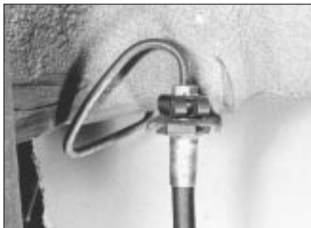
11.2 Rigid pipe-to-flexible hose connection
