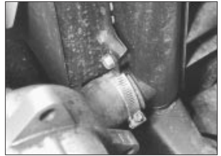
2.4b Radiator bottom hose connection - 1.8 litre
