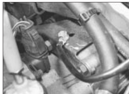
5.8c Earth strap to gearbox
