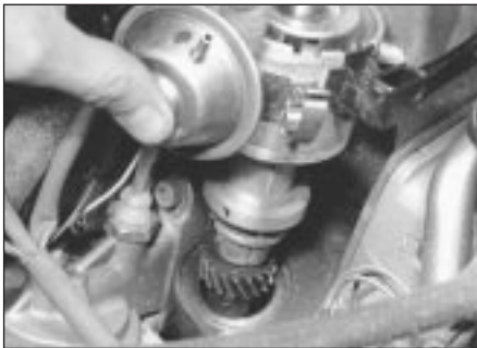
6.6a Distributor removal - 1.8 litre engine
