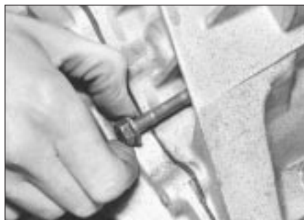
6.6a Undo securing bolts (recessed bolt shown) . . .
