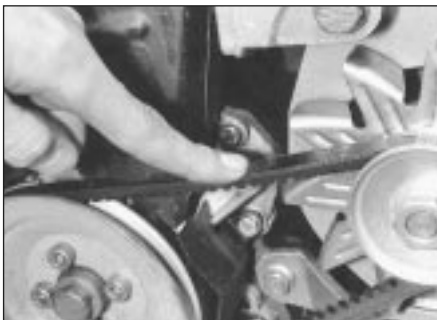
13.2 Checking alternator drivebelt tension
