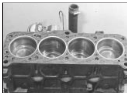
34.2 Cylinder head gasket located on block
