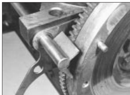
13.2 One method of holding the flywheel stationary
