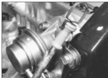
8.1c Engine dipstick and tube
